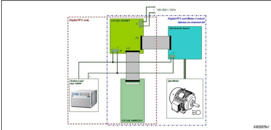
1. Connect the AC power source to pins 1 and 3 of the J7 connector of the STEVAL-ISF002V1.
