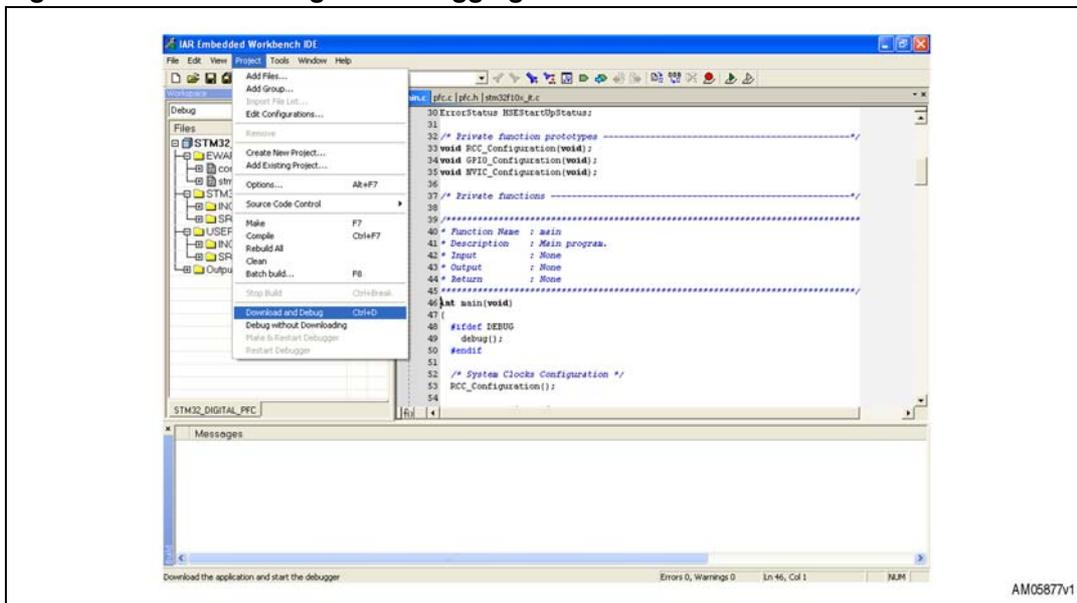
As soon as the download is complete you can unplug the J-LINK probe. Once you have reset the STM32, the control board will be ready for you to try out the demonstrator.
