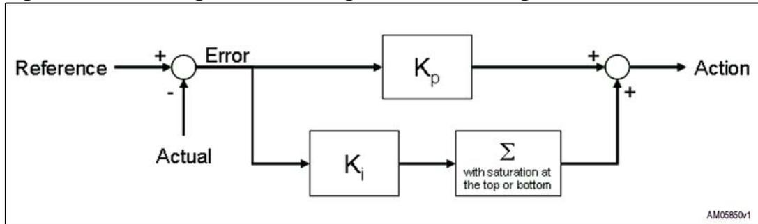
By means of a "voltage error compensator" it is possible to follow the target of the output voltage. Moreover, its output is used as a scaling factor for the Vac, the latter used as the current reference input for the "current error compensator". The output of this last PI is the actual duty cycle of the PFC power MOSFET.
