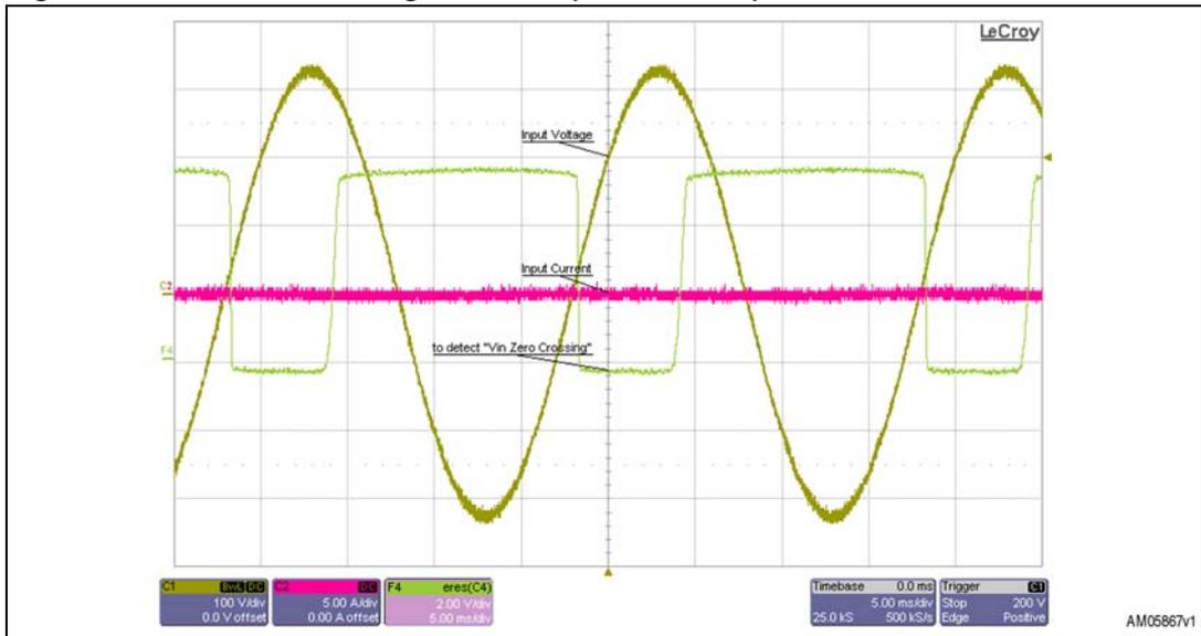
Figure 24. Vin zero crossing detection (with load)
