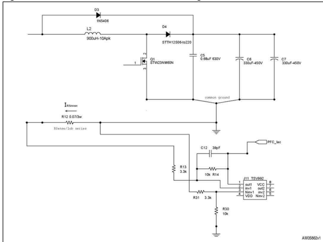
Figure 19. STEVAL-IHM022V1 - PFC current sensing section
