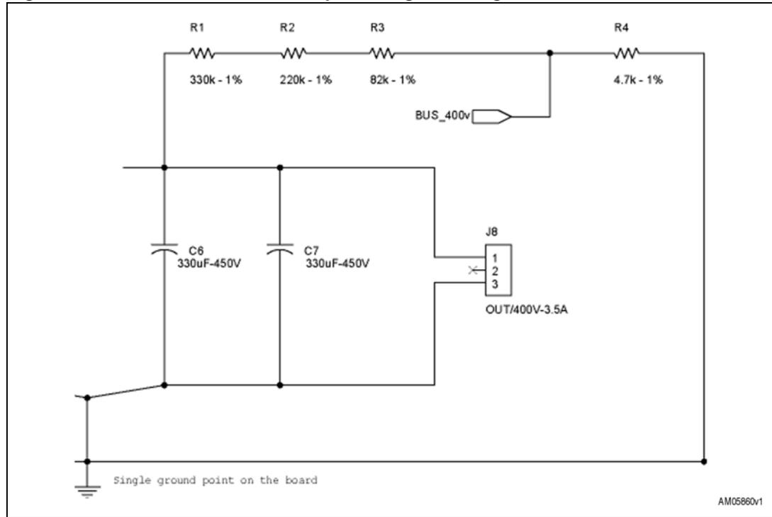
Figure 17. STEVAL-IHM022V1 - output voltage sensing section
