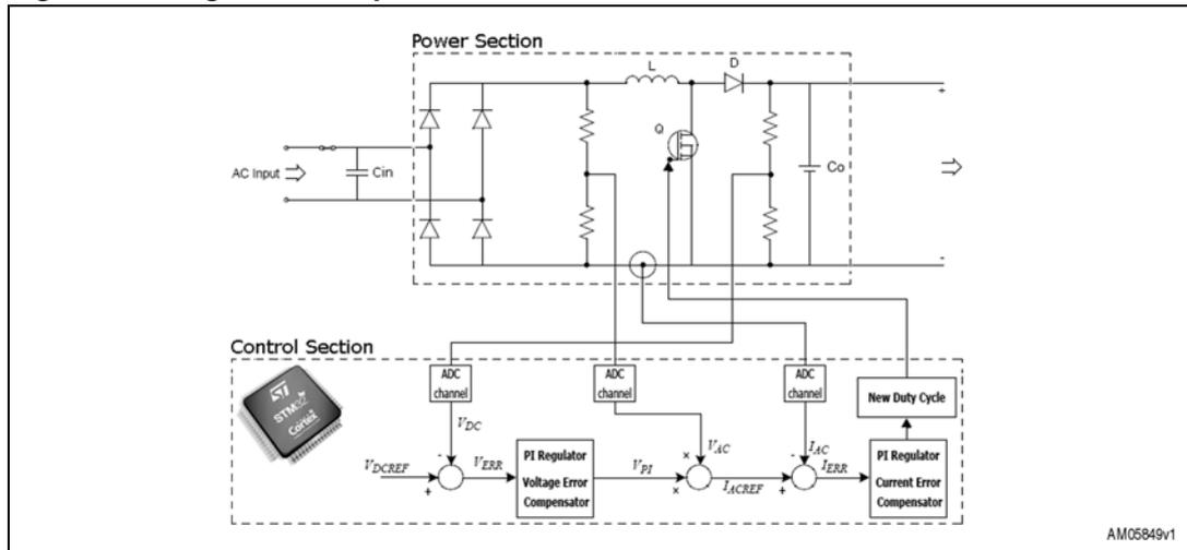
Note: The power section is composed of the STEVAL-ISF002V1 (covered in this user manual). The control section is composed of the STEVAL-IHM022V1 (covered in UM0686).
