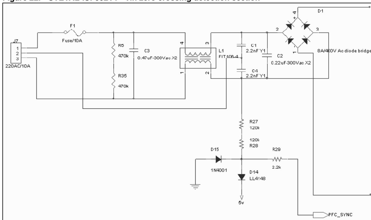
From PFC\_SYNC, information can be obtained on the zero crossing of the input voltage as shown in *Figure 23*.
