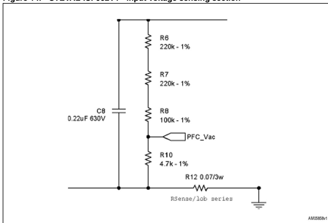
Figure 15. STEVAL-IHM022V1 - input voltage sensing section
