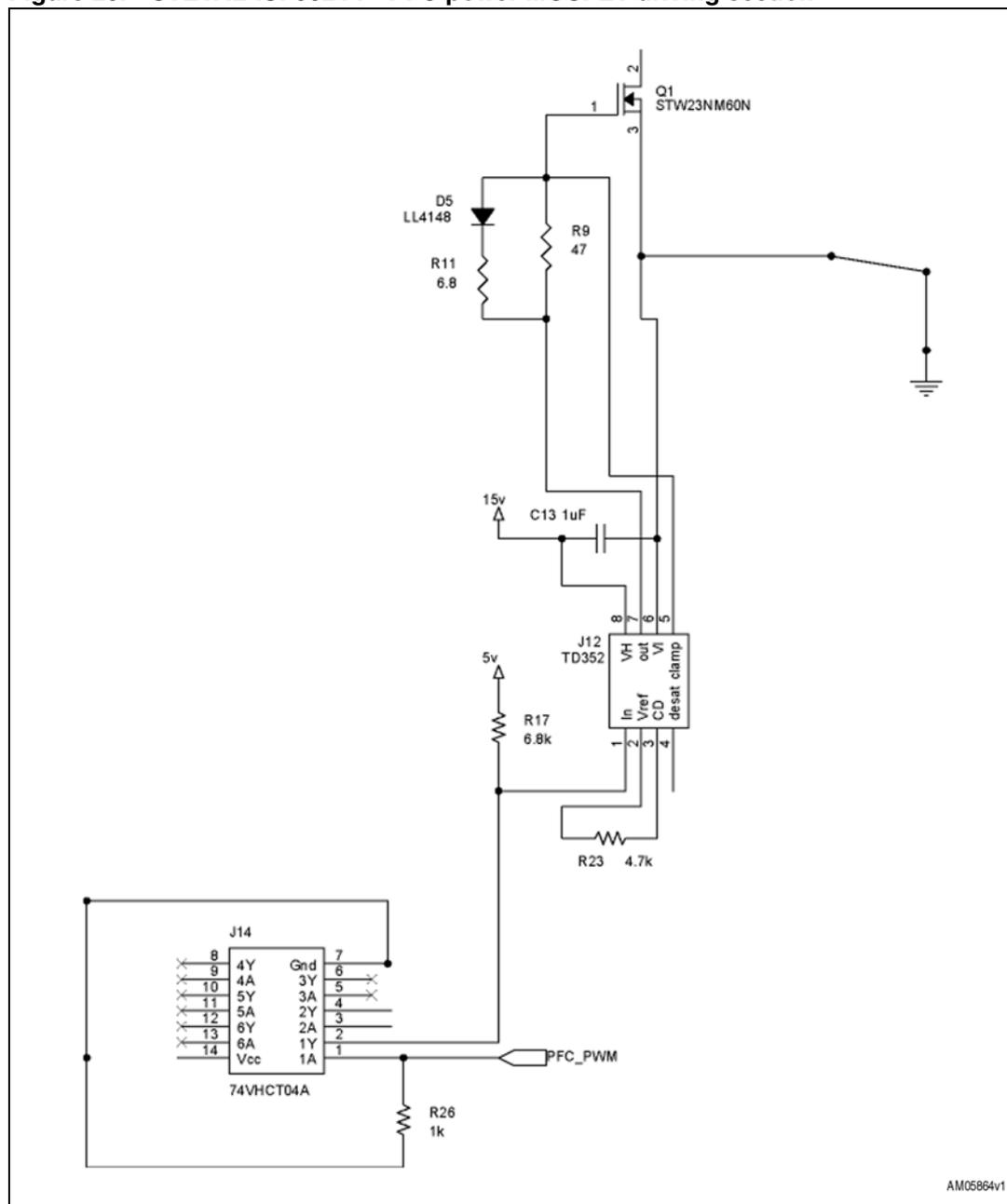
The PFC\_PWM provided by the MCU is inverted and sent to the MOSFET driver TD352.
