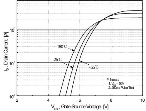
Figure 2. Transfer Characteristics
