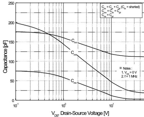
Figure 5. Capacitance Characteristics
