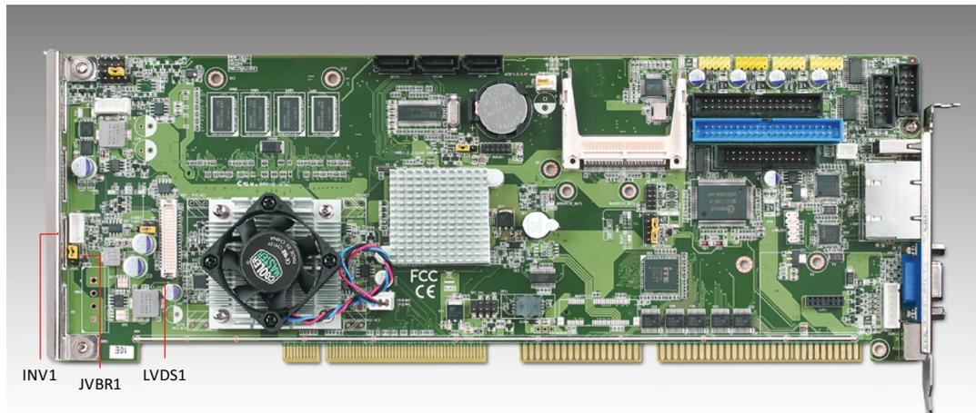
LVDS1 consists of a 40-pin connector which can support 18-bit single channel LVDS with resolution up 1366 x 768. The LCD inverter is connected to INV1 via a 5-pin connector to provide power to the LCD display. JVBR1 provides inverter voltage selection: close pins 1, 2 for 3.3V power input inverter; close pins 2, 3 for 5V power input inverter.
