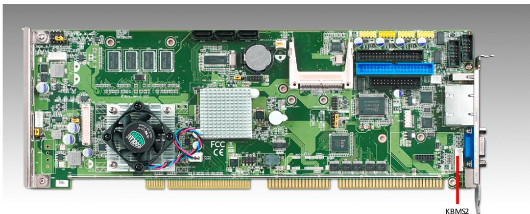
**Figure 2.7 External Keyboard Connector (KBMS2)**
