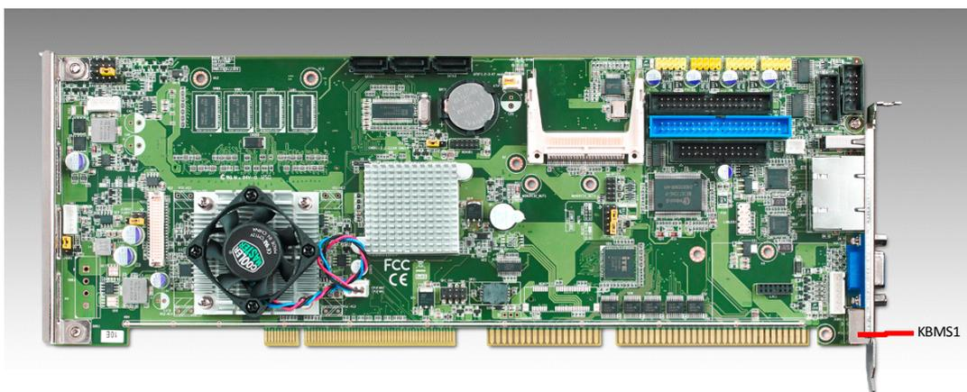
**Figure 2.6 PS/2 Keyboard/Mouse Connector (KBMS1)**
