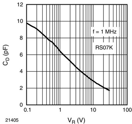
Fig. 5 - Typical Diode Capacitance vs. Reverse Voltage
