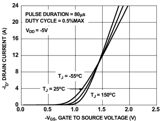
**Figure 5. Transfer Characteristics**
