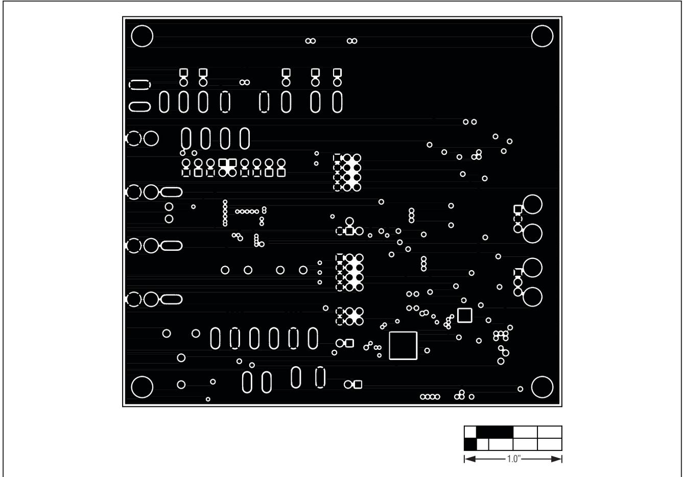
Figure 10. MAX98088 EV Kit PCB Layout—Ground Layer 5
