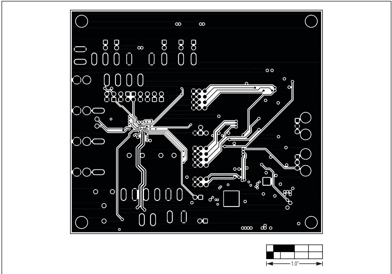
Figure 8. MAX98088 EV Kit PCB Layout—Ground Layer 3
