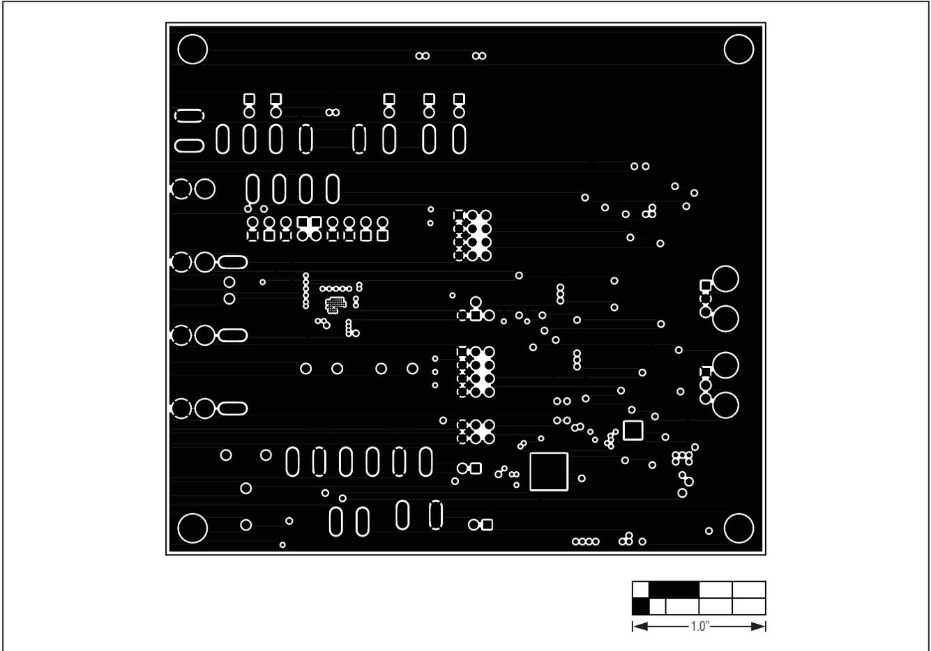
Figure 7. MAX98088 EV Kit PCB Layout—Ground Layer 2
