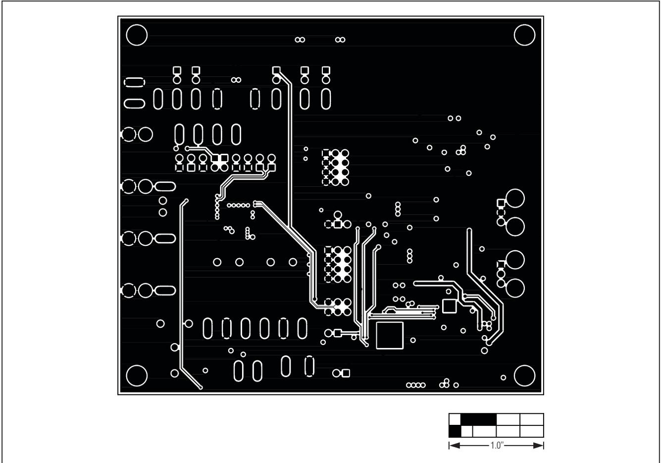
Figure 11. MAX98088 EV Kit PCB Layout—Solder Side
