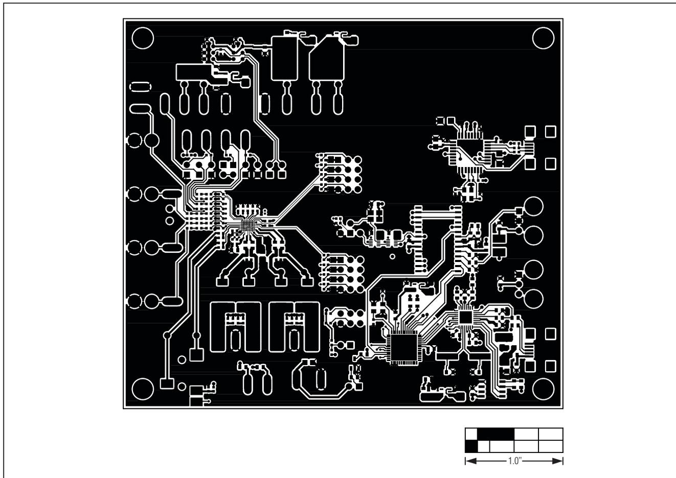
Figure 6. MAX98088 EV Kit PCB Layout—Component Side
