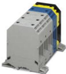
High-current terminal block, Connection method: Screw connection, Number of connections: 10, Number of positions: 5, Cross section: 70 mm<sup>2</sup> - 240 mm<sup>2</sup>, AWG: 2/0 - 500 kcmil, Width: 180 mm, Height: 124 mm, Color: gray/blue/black-yellow, Mounting type: Direct screw connection
