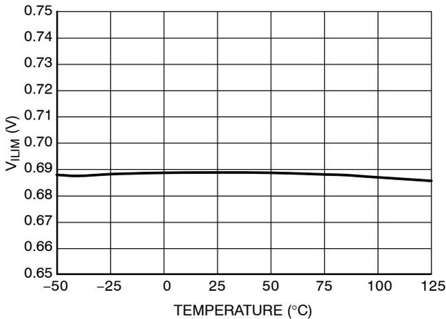
Figure 7. Maximum Internal Current Setpoint
