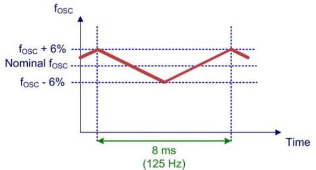
Figure 55. Frequency Modulation of the Maximum Switching Frequency
