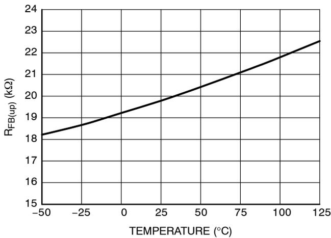
**Figure 13. FB Pin Internal Pull-up Resistor  $R_{FB(up)}$**
