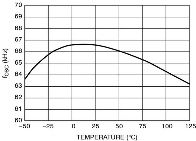
Figure 19. Oscillator  $f_{osc}$  for the 65 kHz Version
