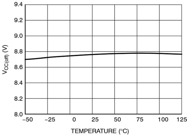
Figure 33.  $V_{CC}$  Turn-off Threshold (UVLO)
