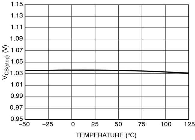
**Figure 9. Threshold for Immediate Fault Protection Activation  $V_{CS(stop)}$**
