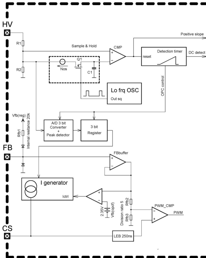
Figure 65. Block Schematic of Overpower Protection Circuit
