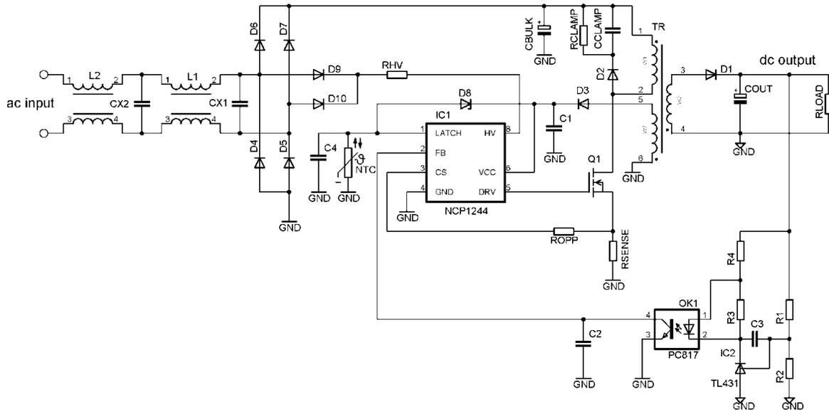
Figure 1. Flyback Converter Application Using the NCP1244
