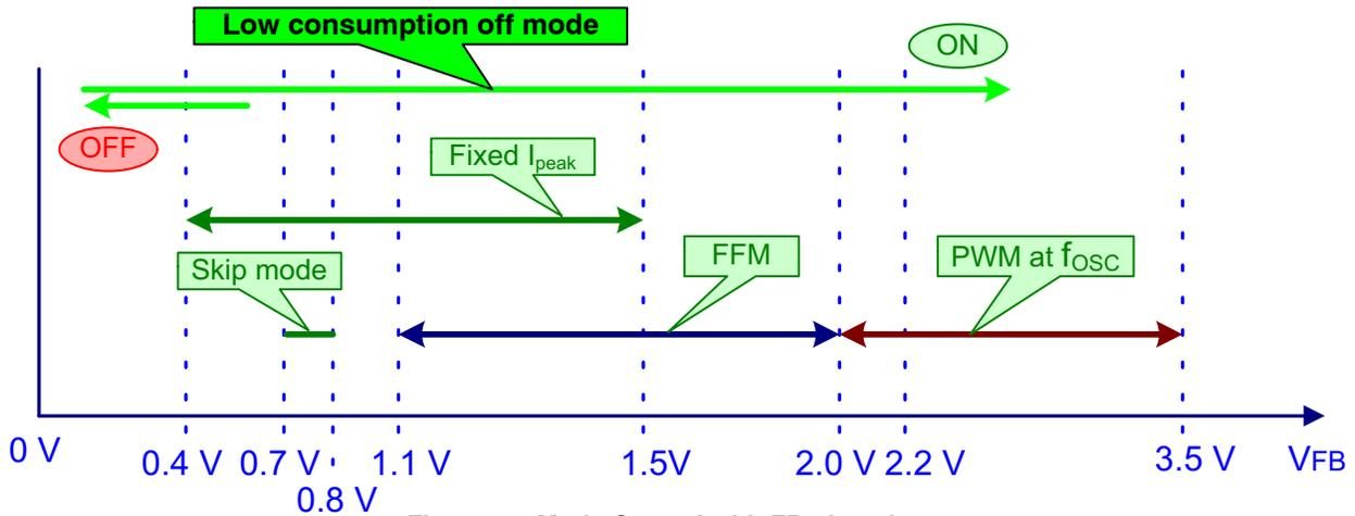
Figure 43. Mode Control with FB pin voltage
