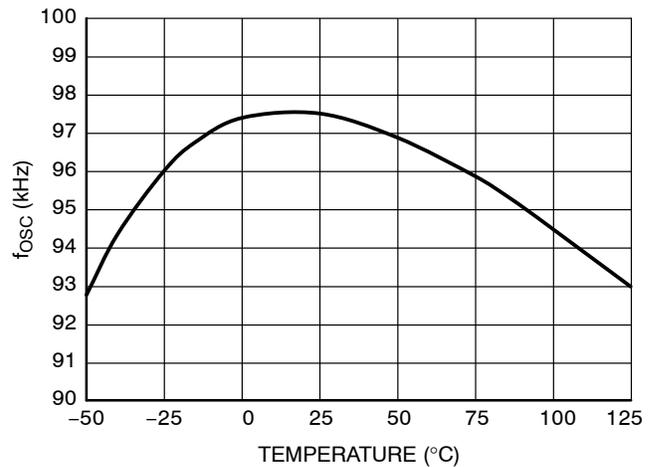
Figure 20. Oscillator  $f_{osc}$  for the 100 kHz Version
