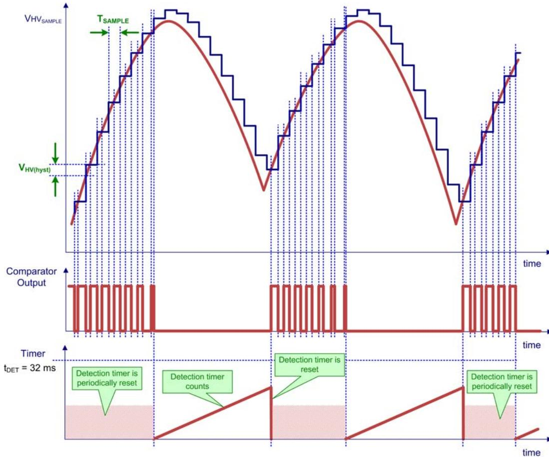
Figure 49. The ac Line Unplug Detector Timing Diagram
