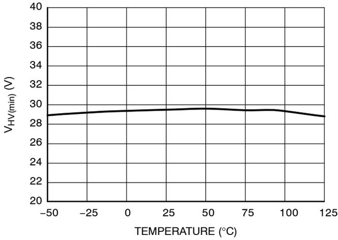
Figure 3. Minimum Current Source Operation
