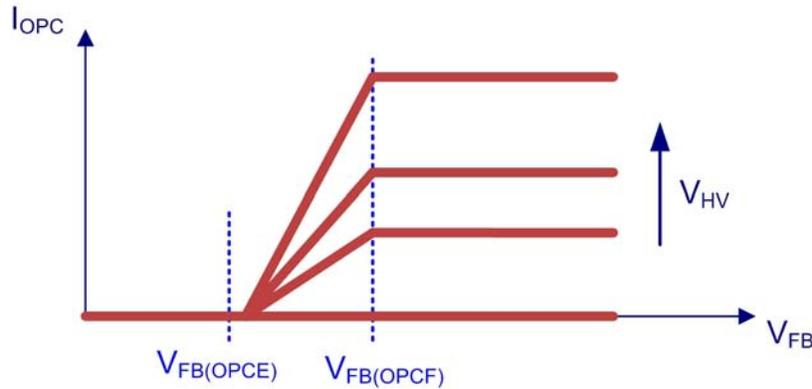
Figure 63. Overpower Protection Current Relation to Feedback Voltage
