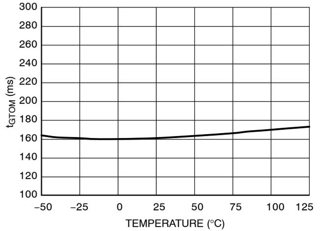
Figure 42. Go To Off Mode Timer Duration  $t_{GTOM}$
