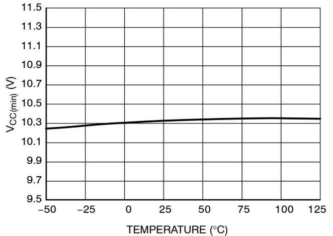
Figure 32. HV Current Source Restart Threshold  $V_{CC(min)}$
