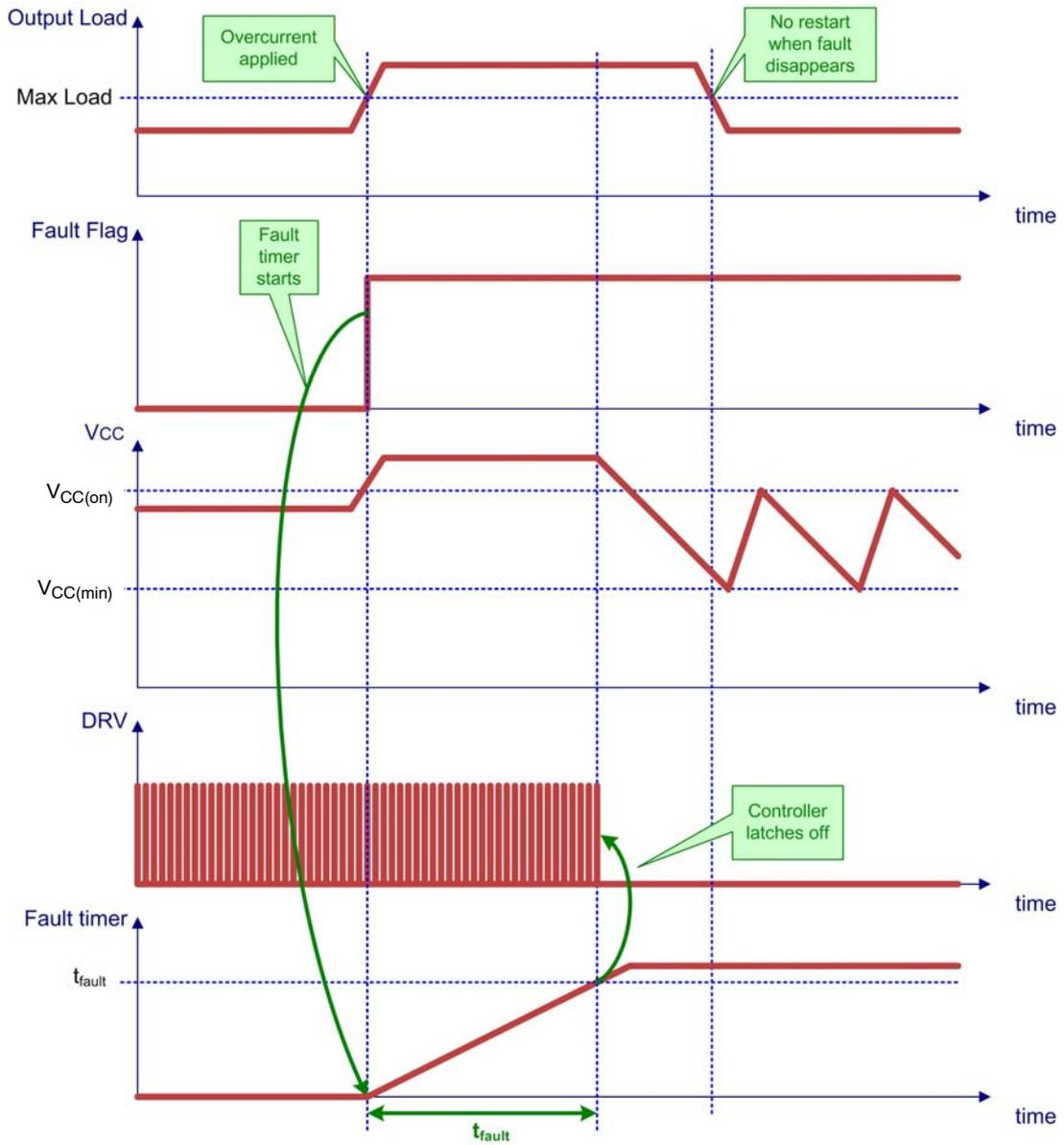
Figure 67. Latched Timer-Based Overcurrent Protection (Option A)
