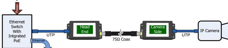
The converters are powered via PoE. PoE compatible cameras will automatically be powered by the Camera Side via UTP. Non-PoE IP camera must use its own power adapter.
