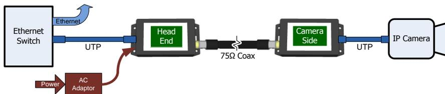
The converters are powered via the power adapter. The IP camera can optionally be powered from the Camera Side Auxiliary power connector, which is at the same voltage as the power adapter (minus any voltage loss in the coax cable – see specifications).
