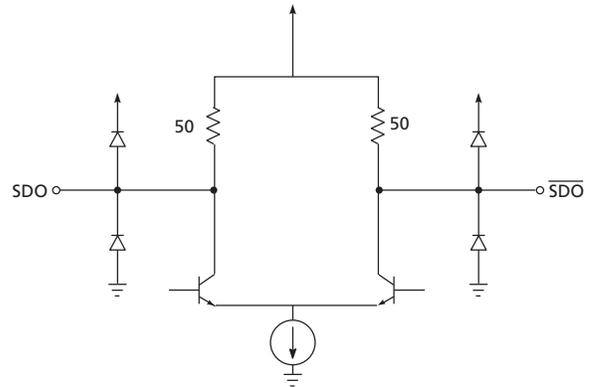
Figure 3-2: Output Circuit
