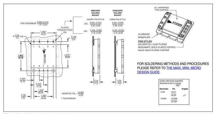
*Figure 13*—*PCB mounting specifications*
