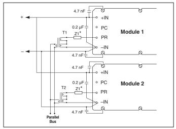
Figure 10 — Transformer-coupled interface.
