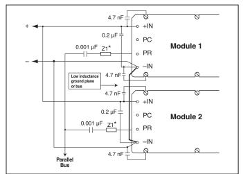
Figure 9 — AC coupled single-wire interface.
