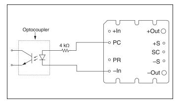
Figure 6 — Isolated on-state indicator.
