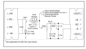
Figure 3 — PC/SC module alarm logic.
