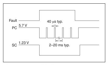
*Figure 5* — *PC/SC module alarm timing.*
