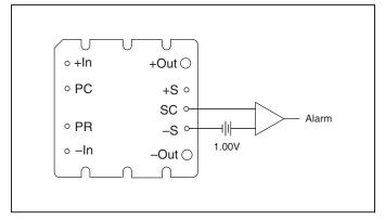
Figure 7 — Secondary side on-state indicator.
