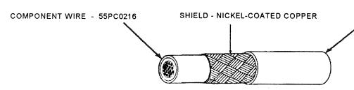
JACKET - RADIATION-CROSSLINKED, MODIFIED ETFE
