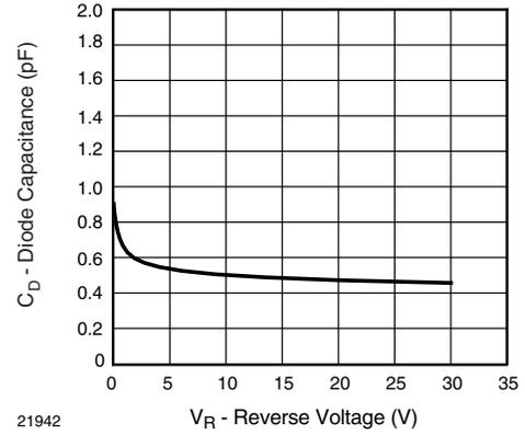
Fig. 6 - Diodes Capacitance vs. Reverse Voltage
