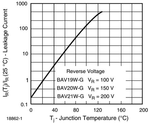
Fig. 5 - Leakage Current vs. Junction Temperature
