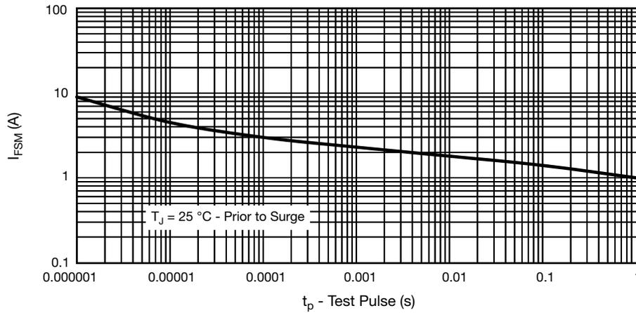
Fig. 7 - Non-Repetitive Peak Forward Current vs. Pulse Duration
