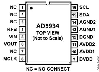
Figure 3. Pin Configuration
