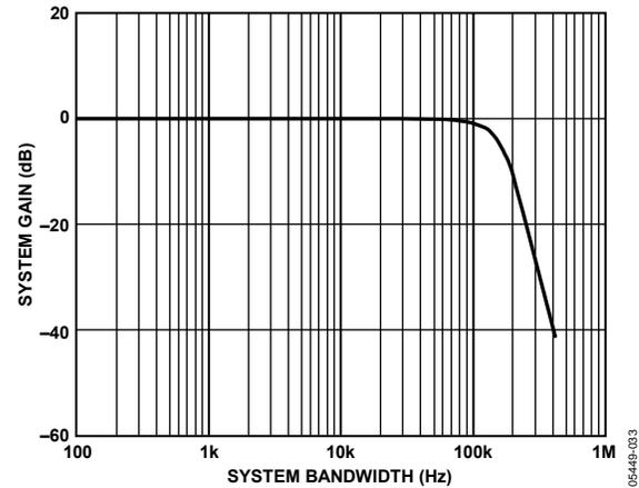
Figure 33. Typical AD5934 System Bandwidth
