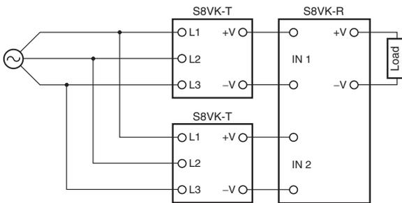
For 960 W, always connect diodes to the output sides of the two Power Supplies as shown in the following diagram.
