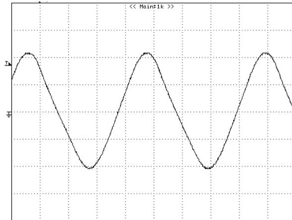
**Figure 25** – Ripple of a Linear adaptor, 115 VAC
