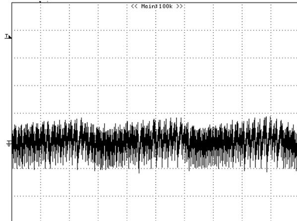
**Figure 23** – Ripple, 115 VAC, Full Load.
