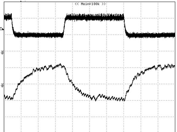
**Figure 19** – Transient Response, 230 VAC, 50-100-50% Load Step.
