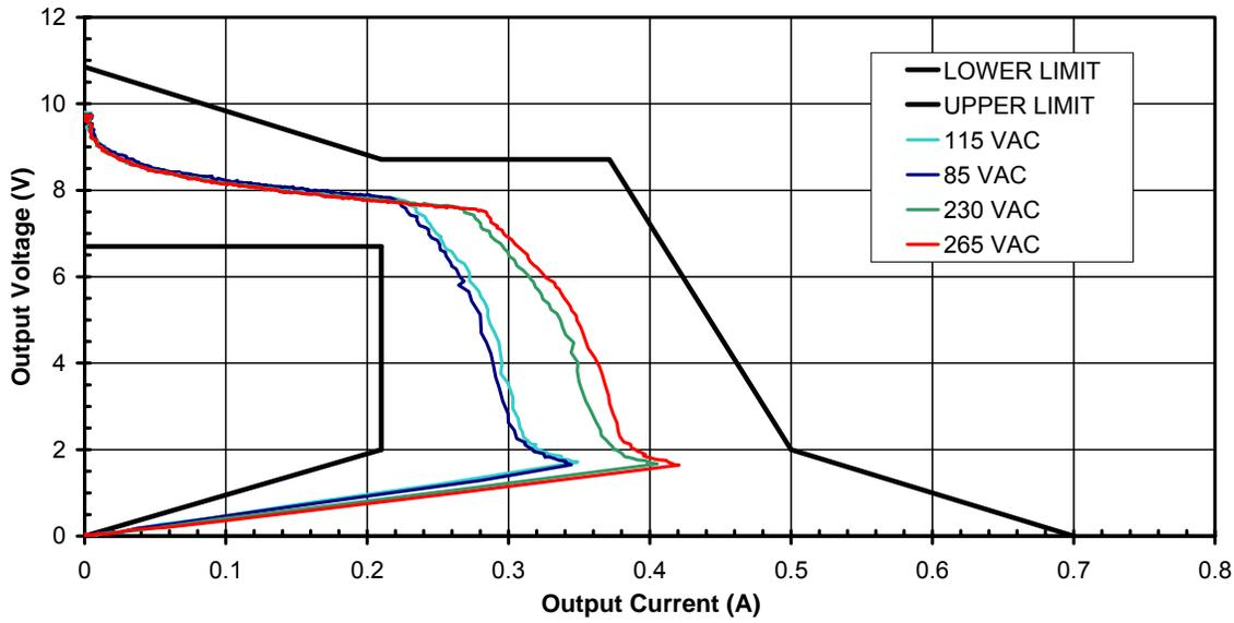
Figure 10 – Output VI Curve, Room Temperature.
