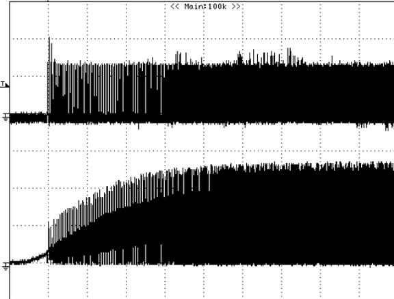
**Figure 16** – 85 VAC Input and Maximum Load.
