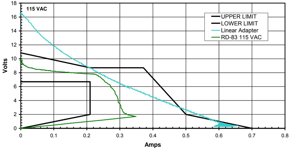
Figure 2 – Output Characteristic Comparison and Limits.
