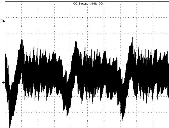
**Figure 22** – Ripple, 85 VAC, Full Load.
