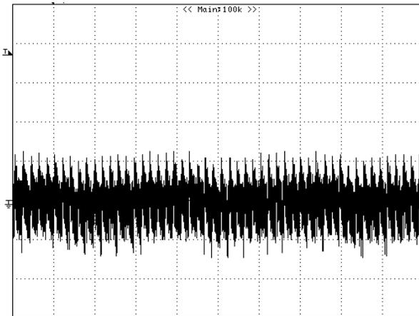
**Figure 24** – Ripple, 230 VAC, Full Load.
