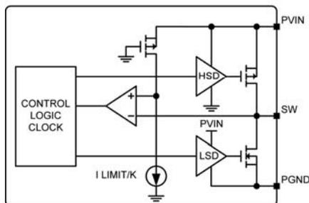
Figure 7. Current-Limit Detail
