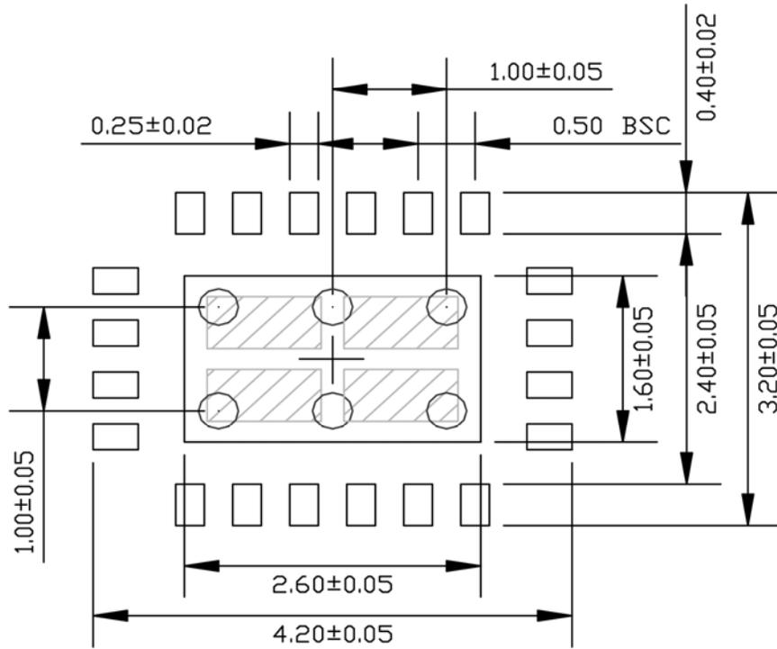
Red circle indicates Thermal Via. Size should be .300-.350 mm in diameter, 1.00 mm pitch and should be connected to GND plane for maximum thermal performance.
