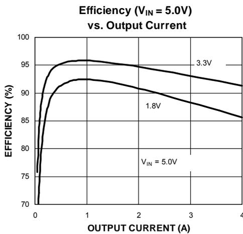
Figure 2. Efficiency Curve
