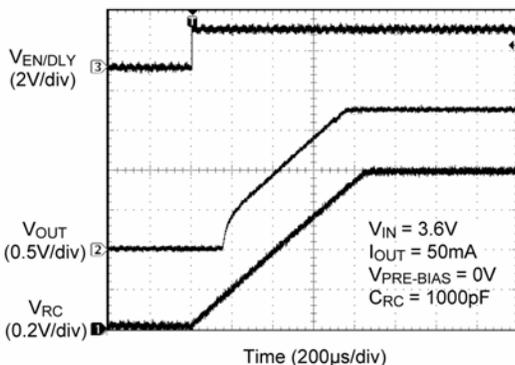
**Figure 3. EN Turn-On Time – Normal Start-Up**
