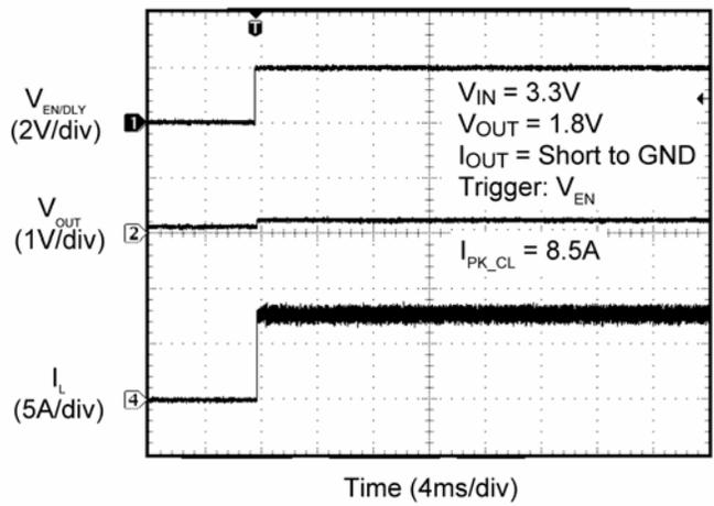
**Output Current Limit Threshold**
