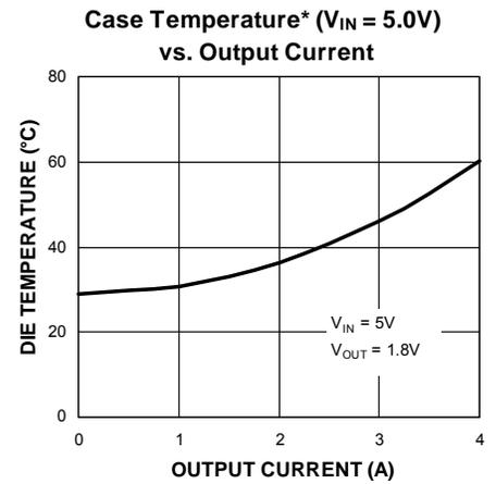
**Die Temperature\*** : The temperature measurement was taken at the hottest point on the MIC22405 case and mounted on a five-square inch PCB (see *Thermal Measurements* section). Actual results will depend upon the size of the PCB, ambient temperature, and proximity to other heat-emitting components.
