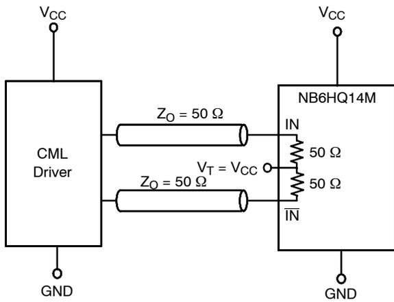
Figure 15. Standard 50 Ω Load CML Interface
