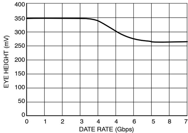
**Figure 4. NB6HQ14M Eye Height vs. Data Rate**
