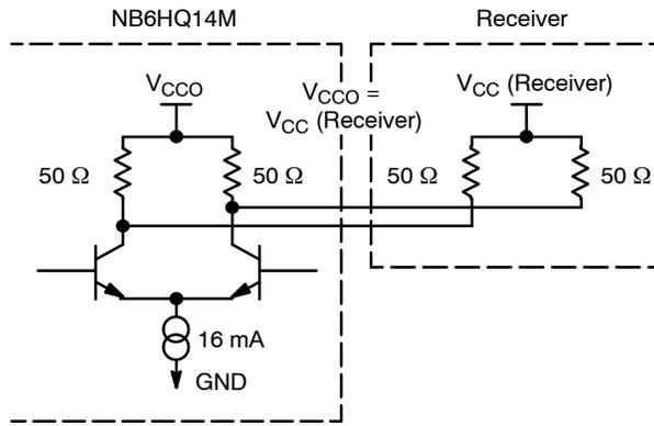
**Figure 18. Typical CML Output Structure and Termination**
