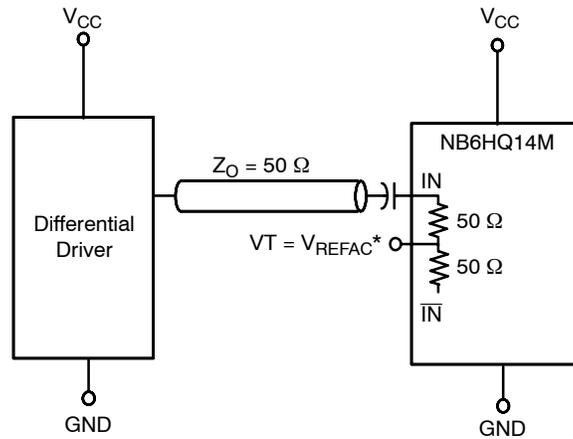
Figure 17. Capacitor-Coupled Single-Ended Interface
