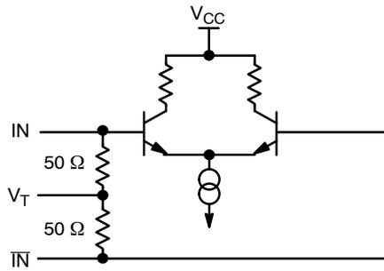
Figure 5. Input Structure
