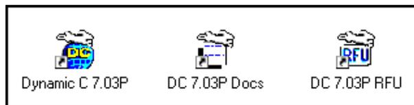
One icon is for Dynamic C, one opens the documentation menu, and the third is for the Rabbit Field Utility, a tool used to download precompiled software to a target system.
