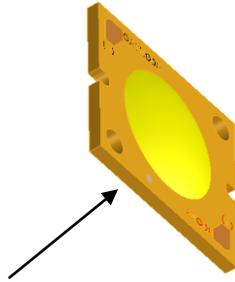
5.0.2 – Apply the M3 or 4-40 screws with 0.2 (MIN) to 0.8 Nm (MAX) of force on each screw
