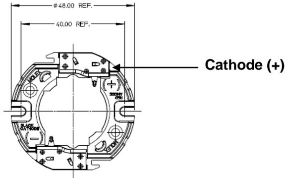
**Note:** wires can be inserted at either end of the Cathode (+) wire trap
