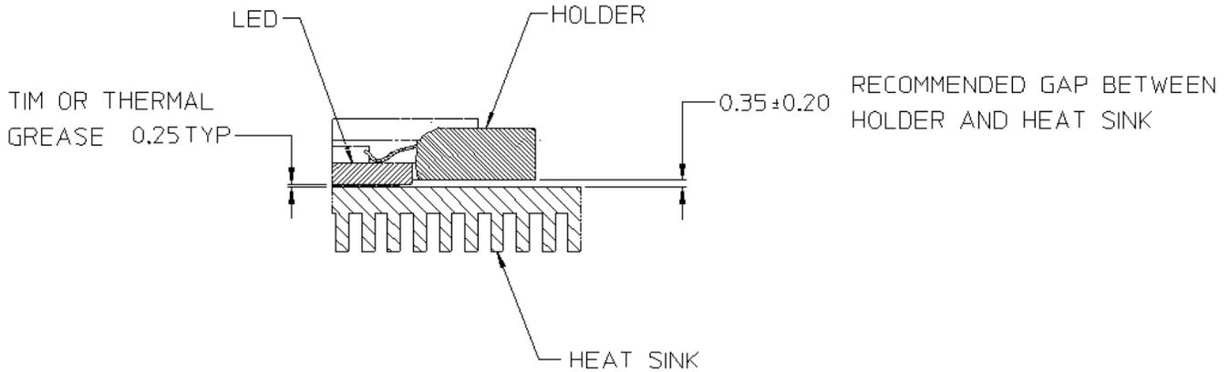
6.0.2 If TIM material exceeds 0.25 mm thickness, the LED holder may tilt excessively when screwed down. It is recommended that the TIM extends to the area below the LED holder as shown below to provide support under the screws.
