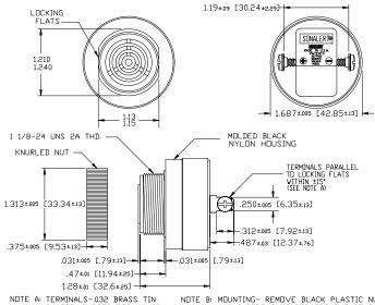
NOTE A: TERMINALS-032 BRASS TIN PLATED, TAPPED FOR #6-32 SCREW. TWD #6-32 NICKEL PLATED BRASS SCREWS INCLUDED, WILL ACCEPT 1/4\* QUICK CONNECT. NOTE B: MOUNTING- REMOVE BLACK PLASTIC NUT AND INSERT THREADED FRONT THROUGH 1.25' HOLE PUNCHED IN PANEL, IF DRIENTATION IS NEDED, NOTE LOCKING FLATS ON DRAWING. SCREW NUT BACK ON. DO NOT OVERTIGHTEN.
