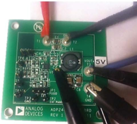
Figure 4. Switch Node Measurement
