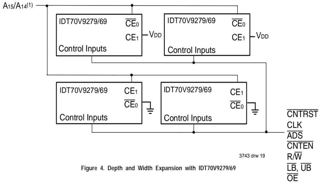
Figure 4. Depth and Width Expansion with IDT70V9279/69
