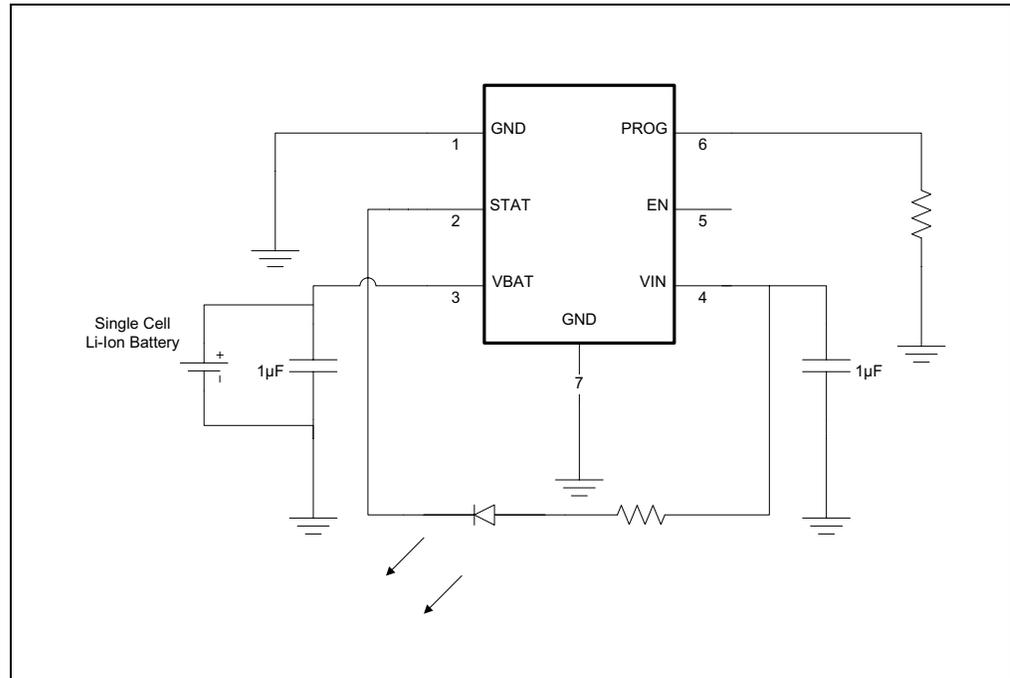
**FIGURE 1-1:** MCP73830L Typical Application Circuit.
