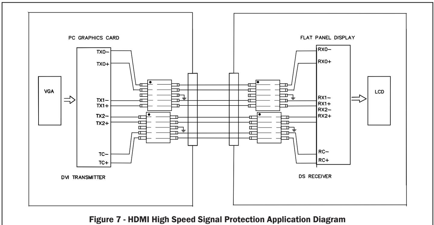
**Figure 7 - HDMI High Speed Signal Protection Application Diagram**
