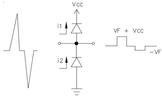
**Figure 4 - “Rail-To-Rail” Protection Topology (First Approximation)**
