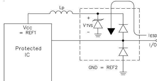
**Figure 6 - Rail-To-Rail Protection Using RailClamp TVS Arrays**
