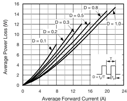
Fig. 2 - Forward Power Loss Characteristics Per Diode
