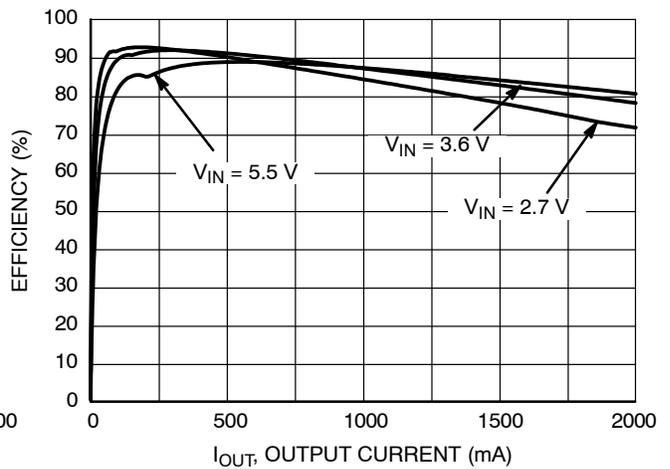
Figure 8. Efficiency vs. Output Current and
