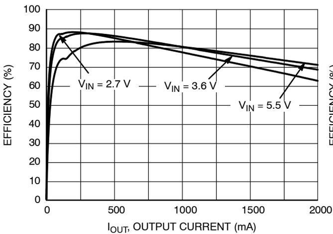
Figure 7. Efficiency vs. Output Current and
