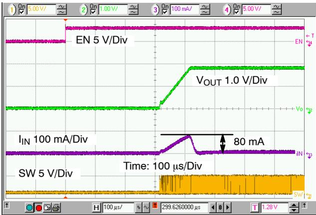
Figure 15. Power Up Sequence and Inrush Current in Input ( $V_{IN} = 3.6\text{ V}$ ,  $V_{OUT} = 1.8\text{ V}$ ,  $I_{OUT} = 0\text{ A}$ ,  $L = 1.0\text{ }\mu\text{H}$ ,  $C_{OUT} = 10\text{ }\mu\text{F}$ )
