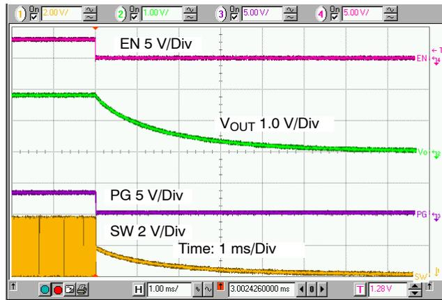
Figure 17. Power Down Sequence and Active Output Discharge ( $V_{IN} = 3.6\text{ V}$ ,  $V_{OUT} = 1.8\text{ V}$ ,  $I_{OUT} = 0\text{ A}$ ,  $L = 1.0\text{ }\mu\text{H}$ ,  $C_{OUT} = 10\text{ }\mu\text{F}$ )
