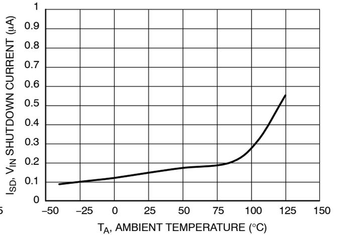
Figure 4. Standby Current vs. Temperature
