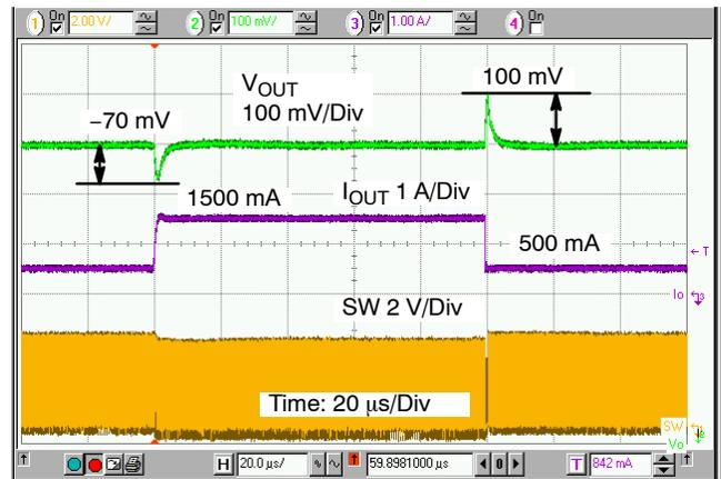
Figure 14. Load Transient Response ( $V_{IN} = 3.6\text{ V}$ ,  $V_{OUT} = 1.8\text{ V}$ ,  $I_{OUT} = 500\text{ mA}$  to  $1500\text{ mA}$ ,  $L = 1.0\text{ }\mu\text{H}$ ,  $C_{OUT} = 10\text{ }\mu\text{F}$ )
