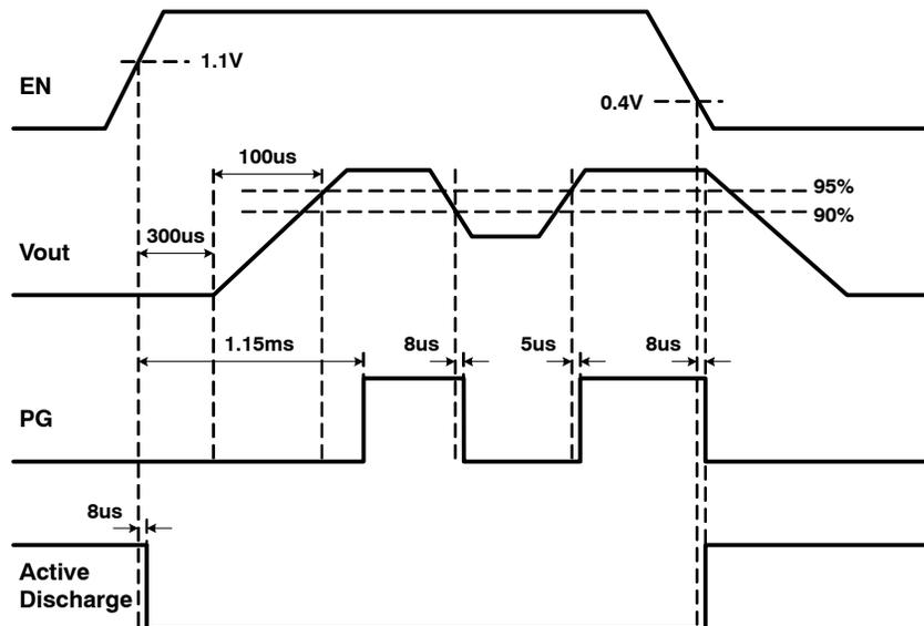
Figure 18. Power Good and Active Discharge Timing Diagram
