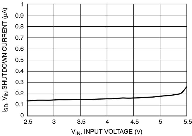
Figure 3. Standby Current vs. Input Voltage
