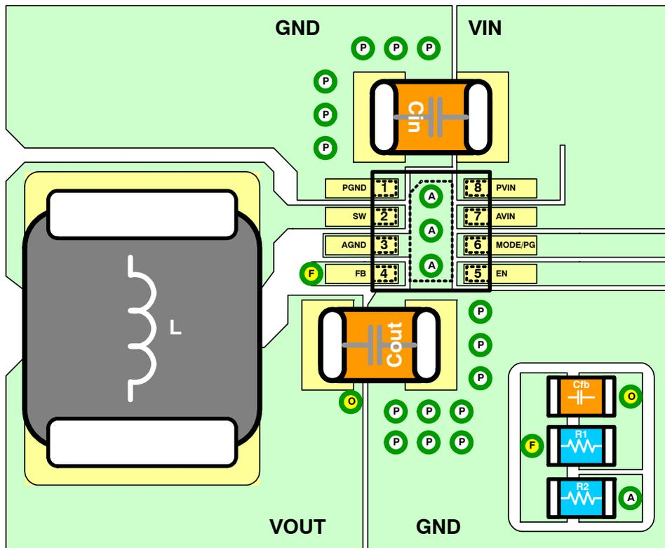
Figure 19. Recommended PCB Layout for Application Boards
