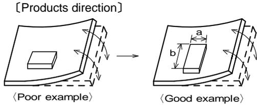
Products shall be located in the sideways direction (Length:  $a < b$ ) to the mechanical stress.
