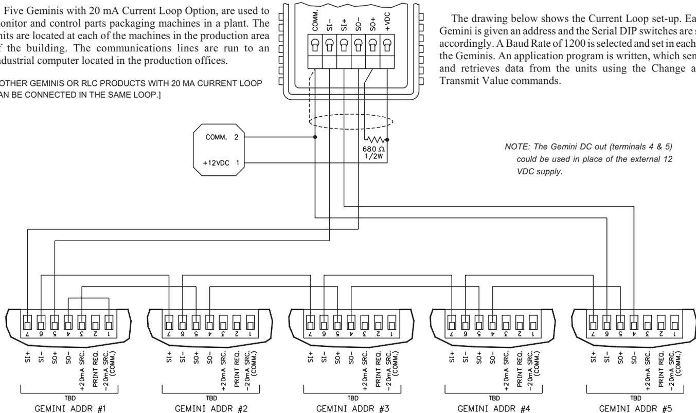
The drawing below shows the Current Loop set-up. Each Gemini is given an address and the Serial DIP switches are set accordingly. A Baud Rate of 1200 is selected and set in each of the Geminis. An application program is written, which sends and retrieves data from the units using the Change and Transmit Value commands.
