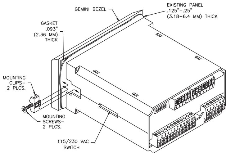
The Gemini is intended to be mounted into an enclosed panel with a gasket to provide a water-tight seal. The unit meets NEMA 4/IP65 requirements for indoor use when properly installed. Two mounting clips and screws are provided for easy installation. Consideration should be given to the thickness of the panel. A panel which is too thin may distort and not provide a water-tight seal. (Recommended minimum panel thickness is 1/8".)
