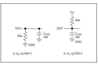
Figure 2. Load Circuits for Disable Time
