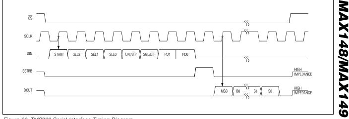
Figure 22. TMS320 Serial-Interface Timing Diagram
