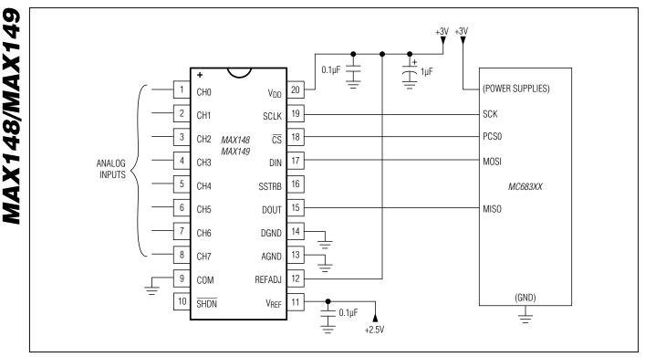
Figure 20. MAX148/MAX149 QSPI Connections, External Reference
