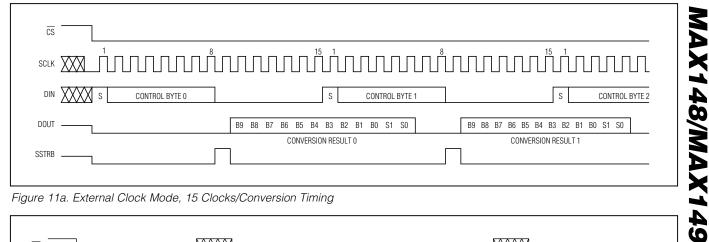
Figure 11a. External Clock Mode, 15 Clocks/Conversion Timing
