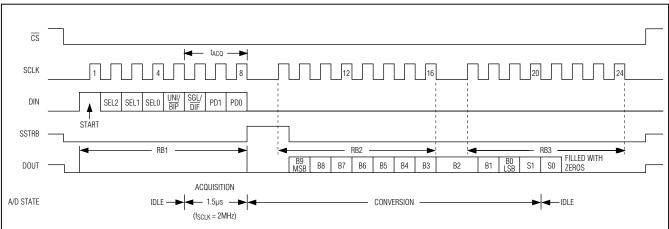
Figure 6. 24-Clock External Clock Mode Conversion Timing (MICROWIRE and SPI-Compatible, QSPI-Compatible with fSCLK ≤ 2MHz)
