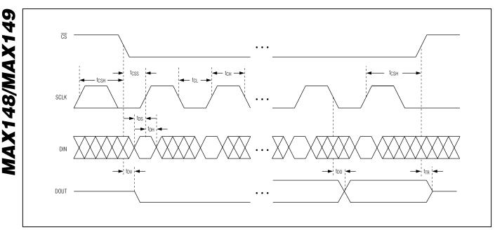
Figure 7. Detailed Serial-Interface Timing
