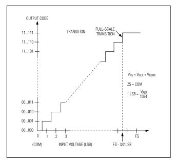
Figure 17. Unipolar Transfer Function, Full Scale (VFS) = V<sub>REF</sub> + V<sub>COM</sub>, Zero Scale (ZS) = COM
