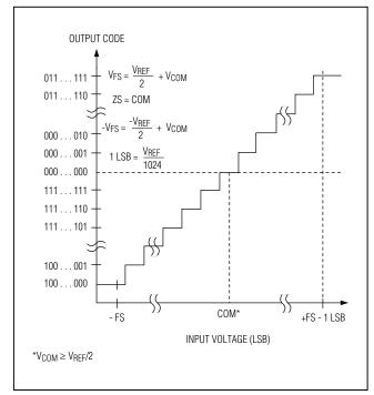
Figure 18. Bipolar Transfer Function, Full Scale (V<sub>FS</sub>) =  $V_{REF}/2$ +  $V_{COM}$ , Zero Scale (ZS) = COM
