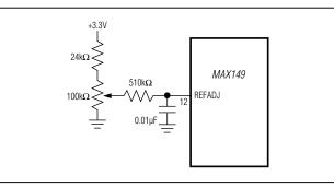
Figure 16. MAX149 Reference-Adjust Circuit
