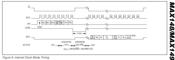
Figure 9. Internal Clock Mode Timing
