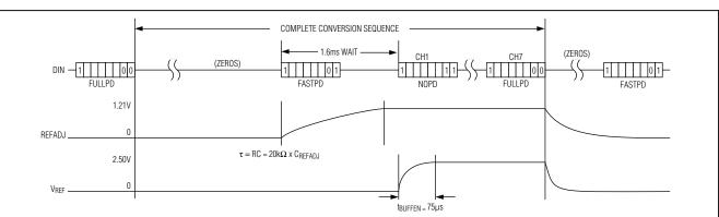
Figure 15. MAX149 FULLPD/FASTPD Power-Up Sequence
