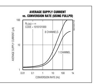
Figure 14a. MAX149 Supply Current vs. Conversion Rate, FULLPD
