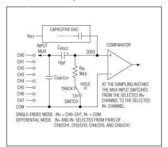
Figure 4. Equivalent Input Circuit
