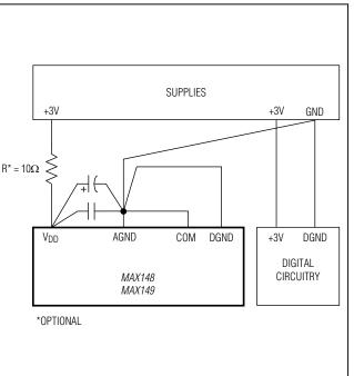
Figure 19. Power-Supply Grounding Connection
