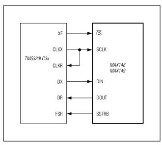
Figure 21. MAX148/MAX149-to-TMS320 Serial Interface
