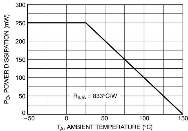
Figure 1. Derating Curve
