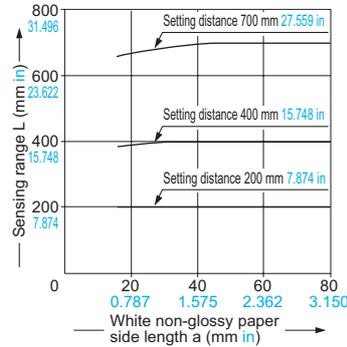
These curves show the characteristics with the maximum sensing range set to 700 mm 27.559 in, 400 mm 15.748 in and 200 mm 7.874 in, with white non-glossy paper (75 × 75 mm 2.953 × 2.953 in).
