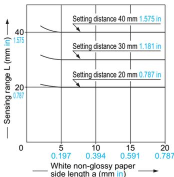
These curves show the characteristics with the maximum sensing range set to 40 mm 1.575 in, 30 mm 1.181 in and 20 mm 0.787 in, with white non-glossy paper (10 × 10 mm 0.394 × 0.394 in).
