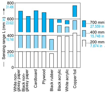
These bars indicate the sensing range with the respective objects when the distance adjuster is set to a sensing range of 700 mm 27.559 in, 400 mm 15.748 in and 200 mm 7.874 in long, respectively, with white non-glossy paper.
