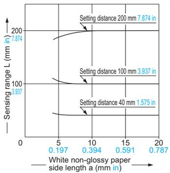
These curves show the characteristics with the maximum sensing range set to 200 mm 7.874 in, 100 mm 3.937 in and 40 mm 1.575 in, with white non-glossy paper (20 × 20 mm 0.787 × 0.787 in).
