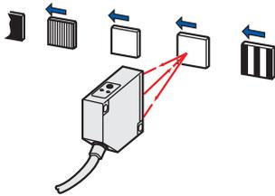
(However, when the background is specular, it may be necessary to change the angle of the sensor.)
