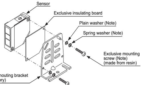
Note: Attached with the exclusive insulating board.
