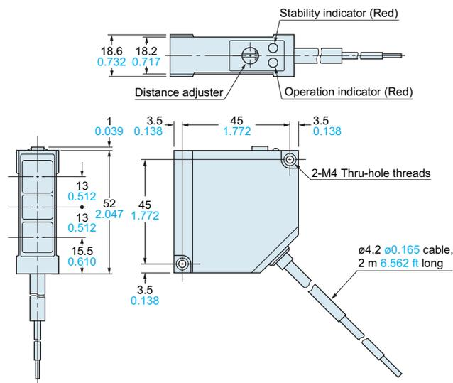
**Assembly dimensions with attached mounting bracket**
