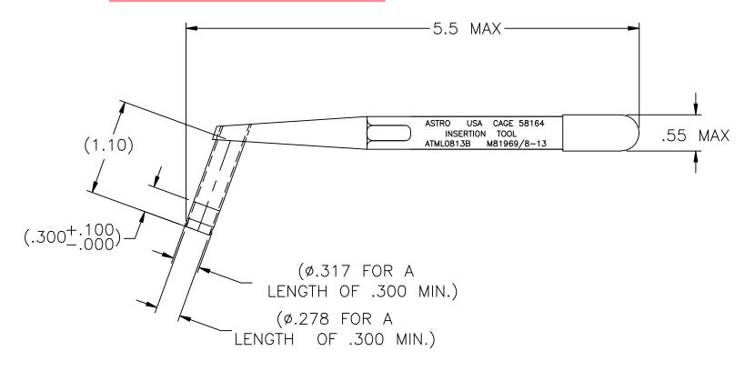
3. WITH TIPS CLOSED AROUND A .2770 +.0000/-.0002  $\phi$  PIN, MAX GAP BETWEEN TIPS TO BE .006.
