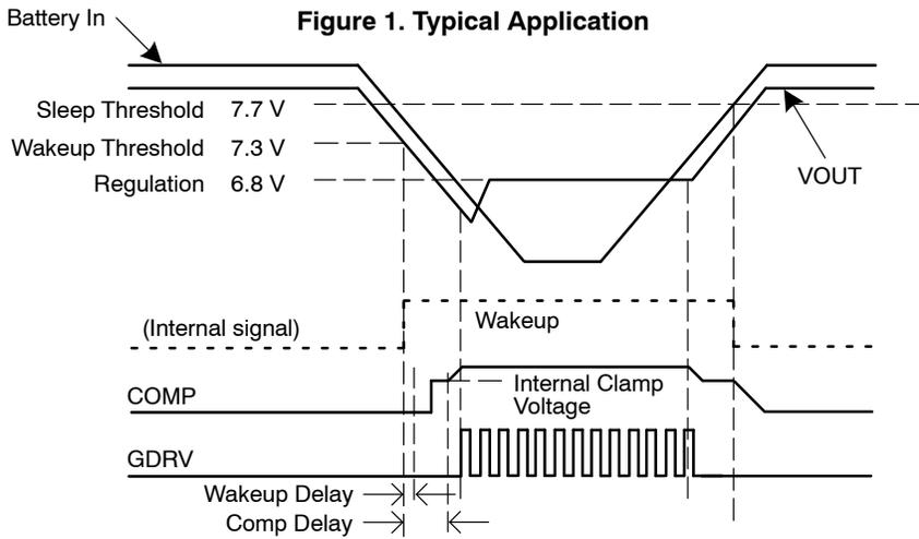
**Figure 2. Functional Waveforms**
