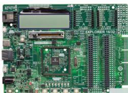
The Explorer 16/32 Development Board is a flexible and convenient development platform for 16-bit PIC24 MCUs, dsPIC® DSCs and 32-bit PIC32 MCUs. The board is driven by the processor Plug-in Modules (PIMs) and facilitates hardware expansion through the use of PICtail™ Plus daughter cards and mikroBUS™ accessory boards. The PIC32 PIMs are supported by the MPLAB Harmony framework featuring various application demos, software libraries and BSPs for faster development.
