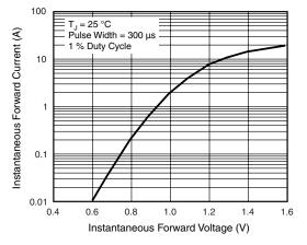
Figure 3. Typical Forward Characteristics Per Diode
