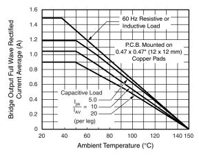
Figure 1. Derating Curve Output Rectified Current
