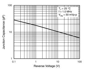
Figure 5. Typical Junction Capacitance Per Diode
