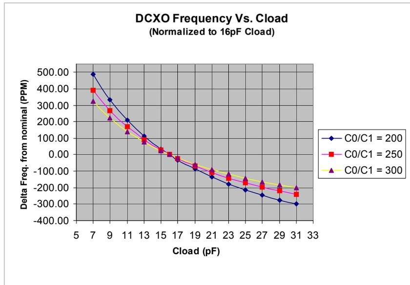
**Table 2. Pullability Range from XTAL with Different C<sub>0</sub>/C<sub>1</sub> Ratio**
