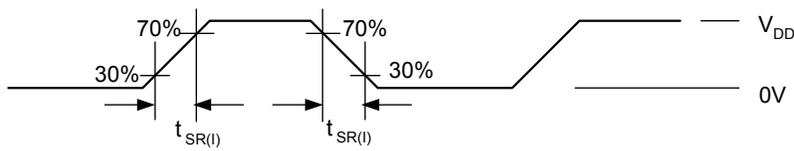
Figure 10. Output Slew Rate
