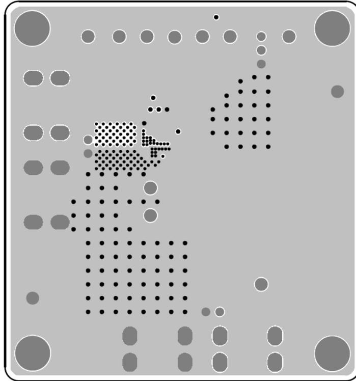
PCB Layout—Inner Side (3<sup>rd</sup> Layer)
