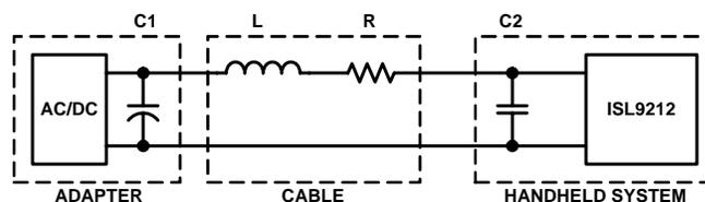
FIGURE 25. EQUIVALENT CIRCUIT FOR THE ISL9212B INPUT
