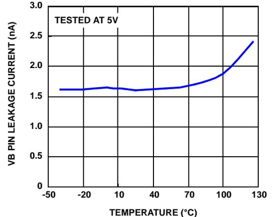
FIGURE 19. VB PIN LEAKAGE CURRENT vs TEMPERATURE
