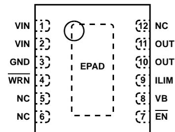
NOTE: EPAD must be electrically connected to the GND pin.
