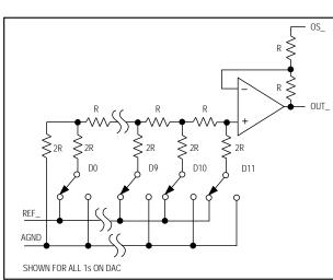
Figure 1. Simplified DAC Circuit Diagram
