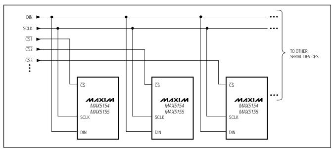
Figure 8. Multiple MAX5154/MAX5155s Sharing a Common DIN Line
