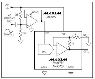
Figure 12. AC Reference Input Circuit
