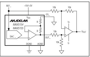
Figure 11. Bipolar Output Circuit
