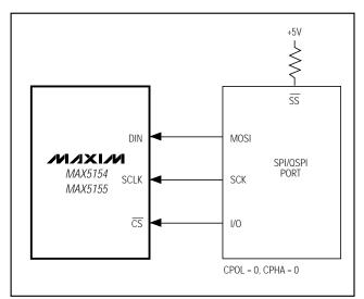
Figure 3. Connections for SPI/QSPI
