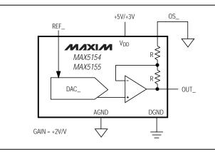
Figure 9. Unipolar Output Circuit (Rail-to-Rail)
