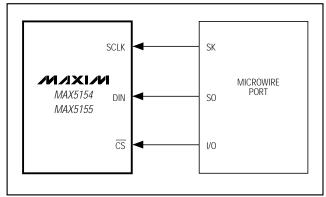
Figure 2. Connections for Microwire
