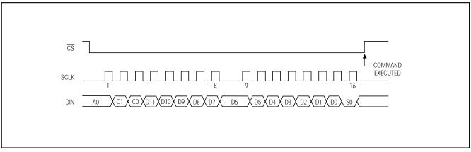
Figure 5. Serial-Interface Timing Diagram
