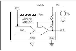
Figure 10. Setting OS\_ for Output Offset
