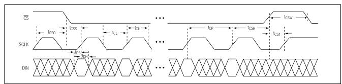
Figure 6. Detailed Serial-Interface Timing Diagram
