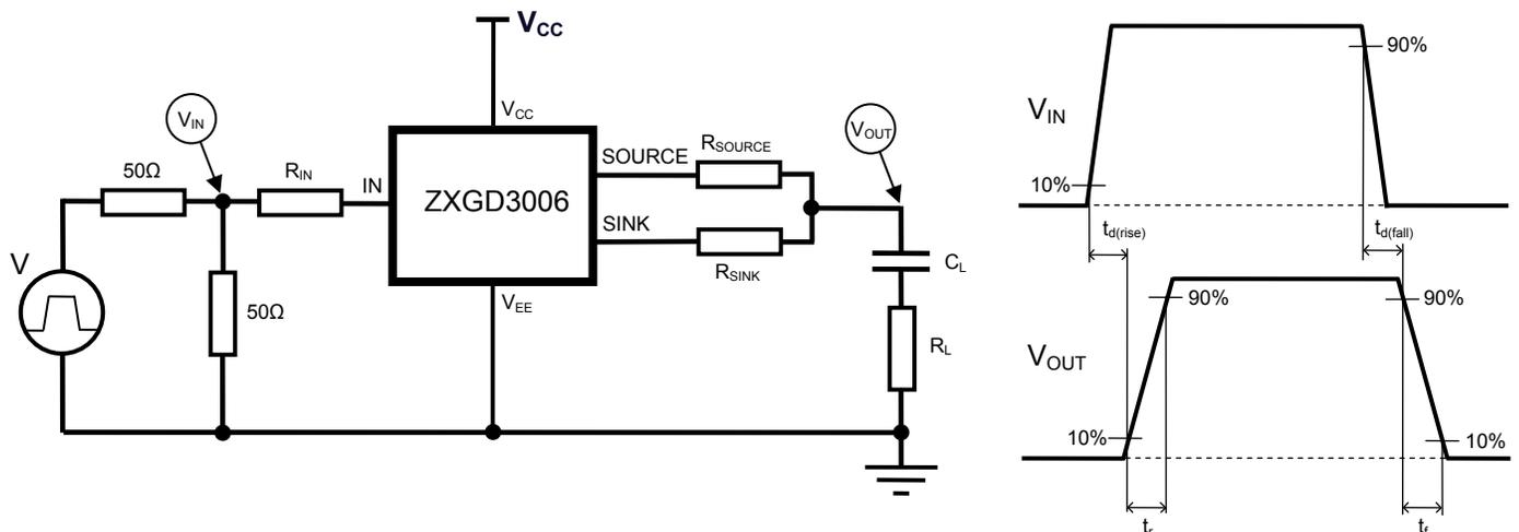
**Typical Switching Characteristics** (@ $T_A = +25^\circ\text{C}$ , unless otherwise specified.)
