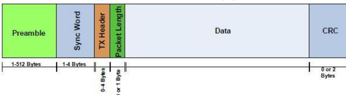
Figure 17. Packet Structure
