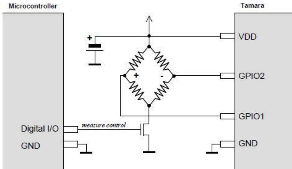
**Figure 25. ADC Differential Input Example—Bridge Sensor**
