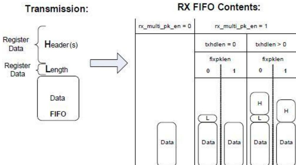
**Figure 20. Multiple Packets in RX Packet Handler**
