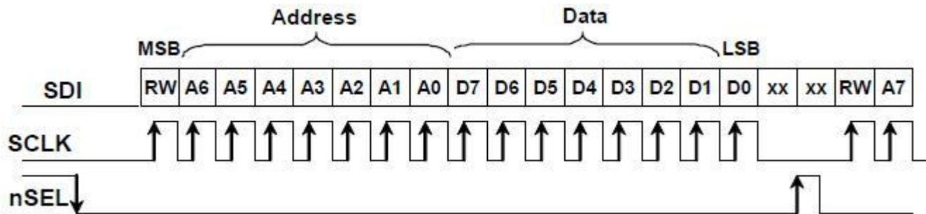
Figure 2. SPI Timing
