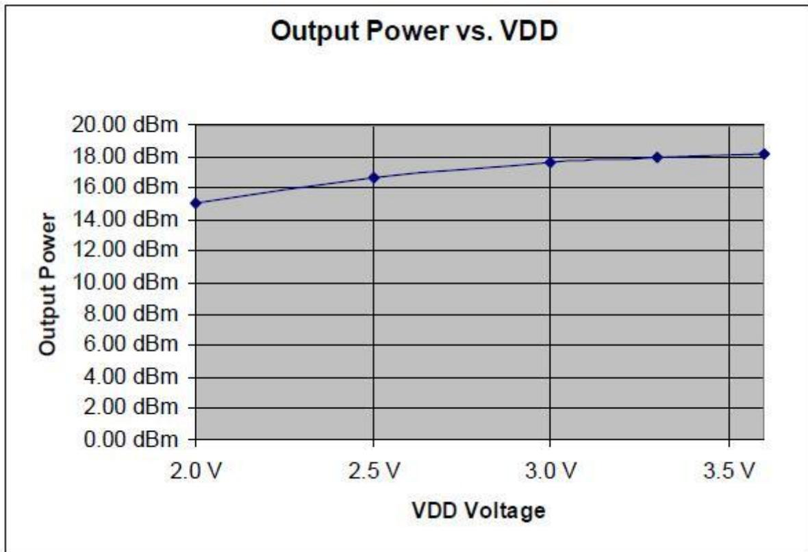
Figure 46. TX Output Power vs. VDD Voltage
