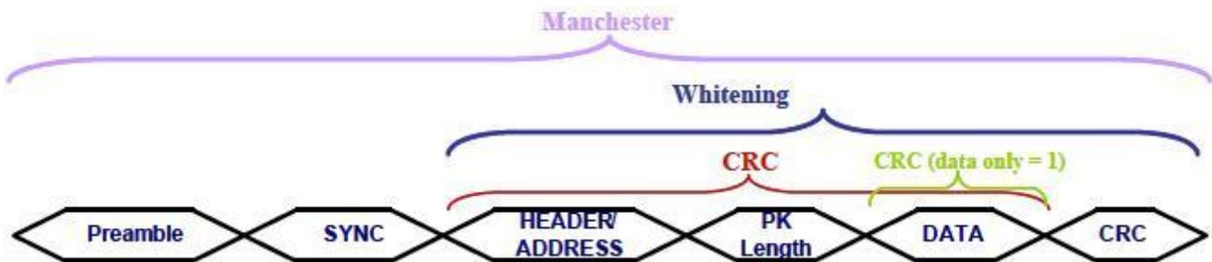
Figure 22. Operation of Data Whitening, Manchester Encoding, and CRC
