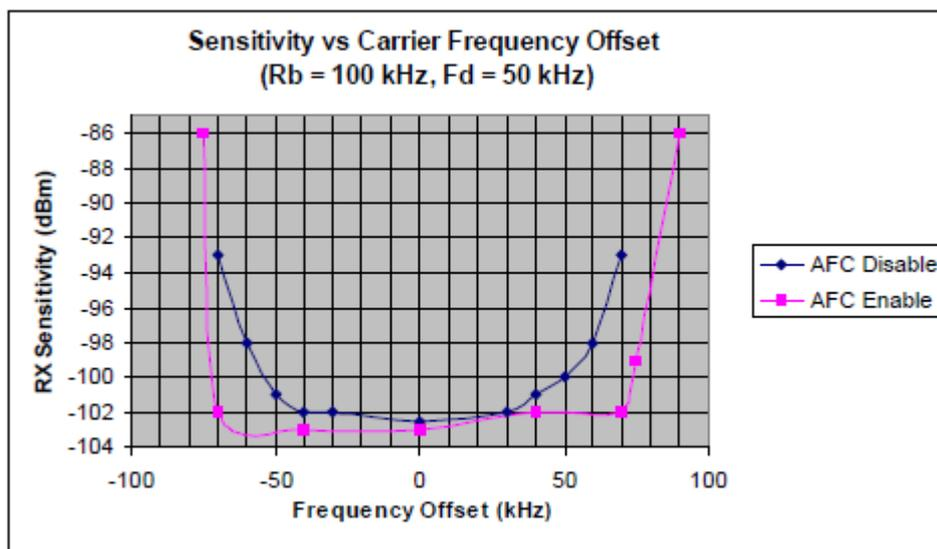
Figure 10. Sensitivity at 1% PER vs. Carrier Frequency Offset
