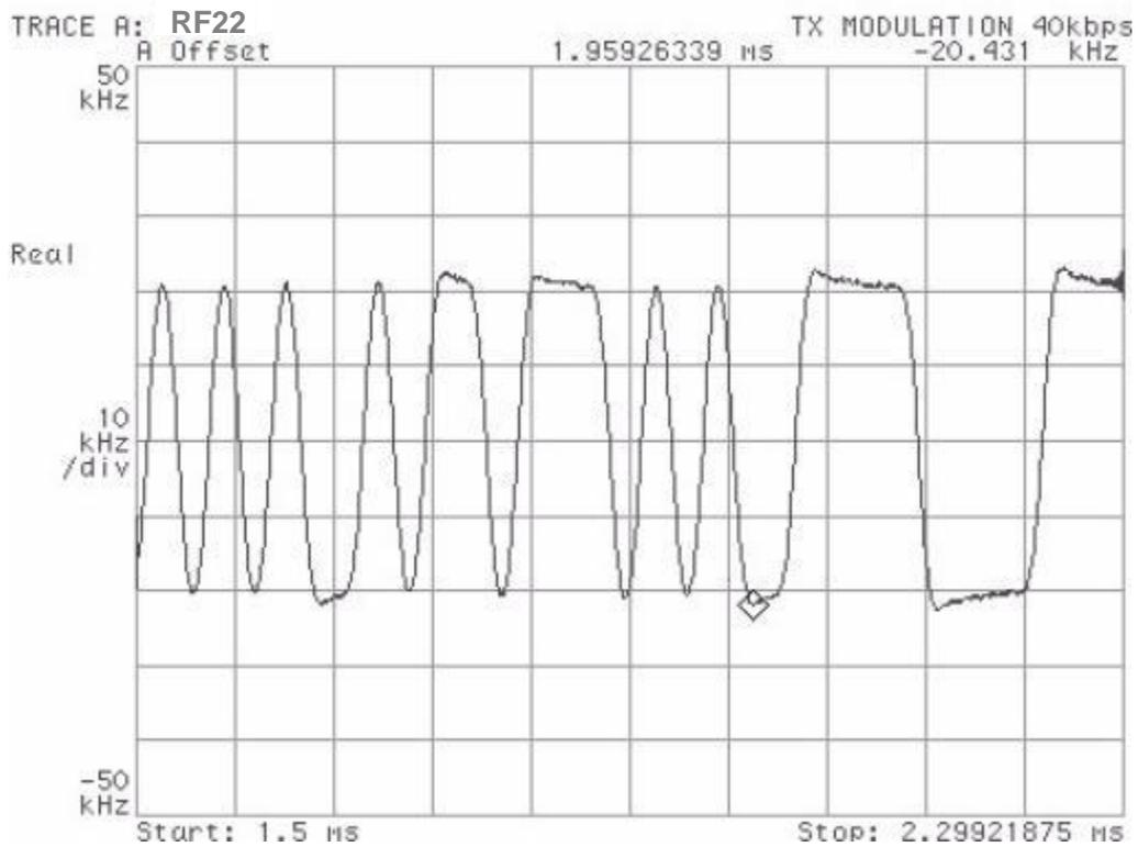
Figure 37. TX Modulation (40 kbps, 20 kHz Deviation)
