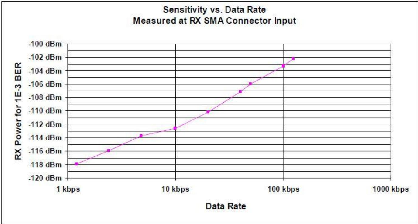
**Note:** Sensitivity is BER measured, GFSK modulation, BT = 0.5, H = 1.
