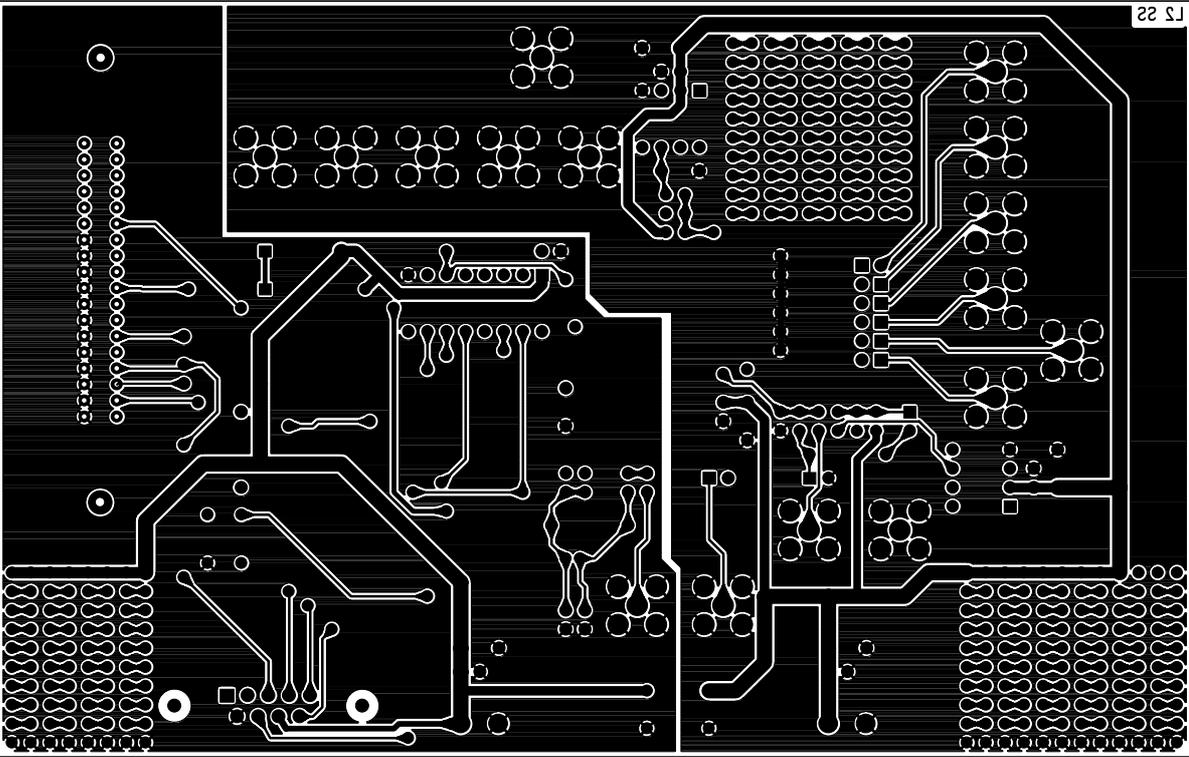
Fig. 20. The Evaluation Board Solder Side Artwork
