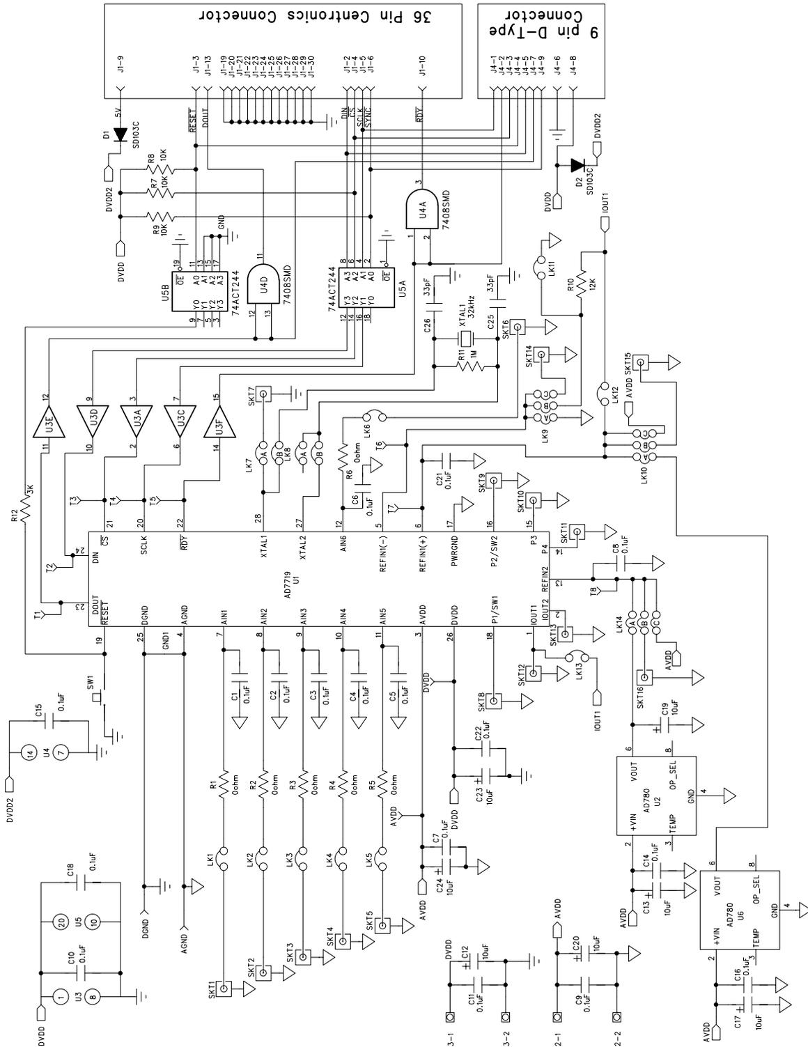
Fig. 17. The Evaluation Board Schematic
