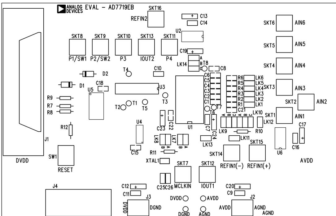
Fig. 18. The Evaluation Board Component Layout Diagram
