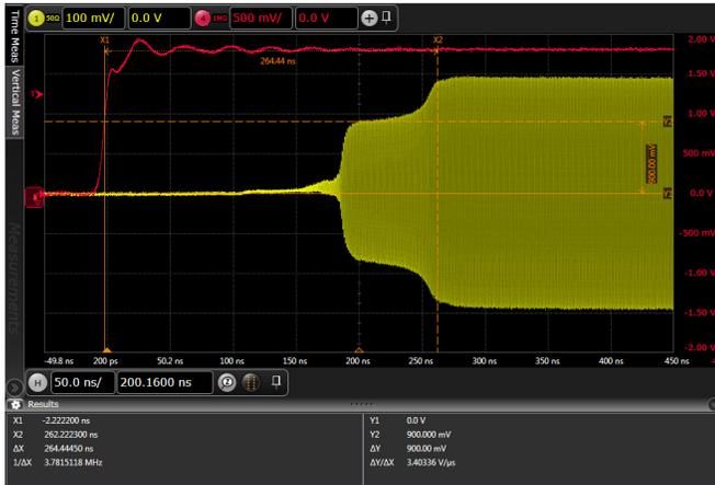
**Figure 17. Switching Time Insertion Loss to Isolation**
