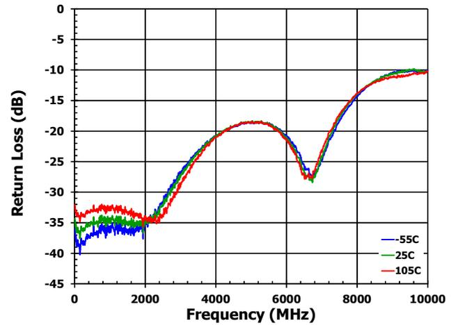
**Figure 8. Return Loss vs. Frequency over Temperature [RF2 Terminated State]**
