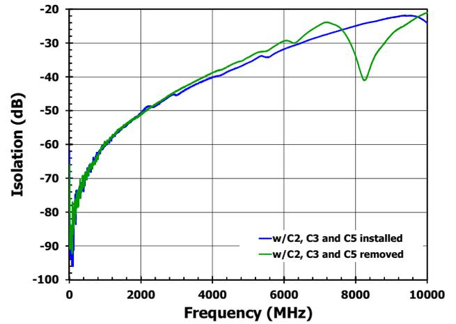
**Figure 12. Return Loss vs. Frequency With and Without Capacitors**
