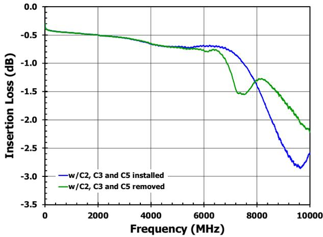
**Figure 11. Isolation vs. Frequency With and Without Capacitors**
