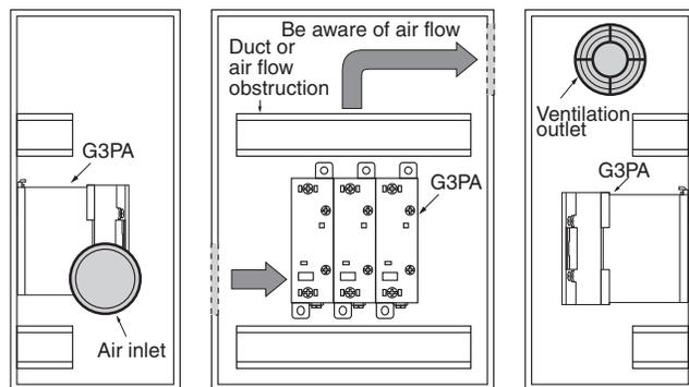
If the air inlet or air outlet has a filter, clean the filter regularly to prevent it from clogging and ensure an efficient flow of air.
