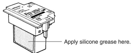
2. Make sure that there is no dust or pieces of wire on the heat sink of the G32A-A or the G3PA.
