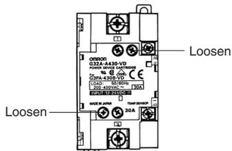
5. Hold the indented part of both the corners to remove the cartridge.
