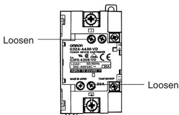
4. Loosen the screws on both the corners.
