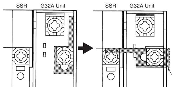
1. When SSR are close mounted, loosen the M3.5 Sems screw on the G32A and flip the linking terminal down.
