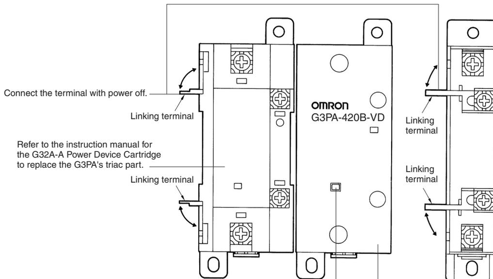
Refer to the instruction manual for the G32A-A Power Device Cartridge to replace the G3PA's triac part.
