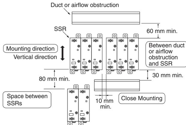
An SSR uses a semiconductor in the output element. This causes the temperature inside the control panel to increase due to heating resulting from the passage of electrical current through the load. To restrict heating, attach a fan to the ventilation outlet or air inlet of the control panel to ventilate the panel. This will reduce the ambient temperature of the SSRs and thus increase reliability. (Generally, each 10°C reduction in temperature will double the expected life.)
