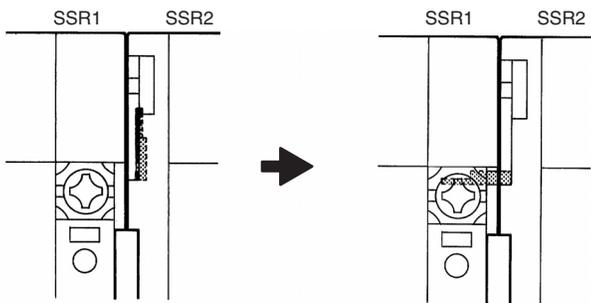
1. When SSRs are close mounted, loosen the M3.5 Sems screw and flip the linking terminal down.
