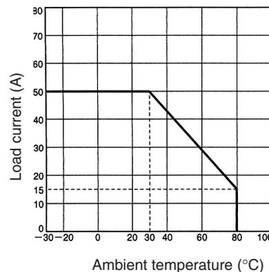
**Note:** Close mounting is possible for a maximum of three Units by reducing the load current by 20%. (A minimum clearance of 10 mm must be provided when mounting four or more Units.)
