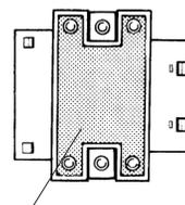
2. Make sure that there is no dust or pieces of wire on the heat sink of the G32A-A or the G3PA.
