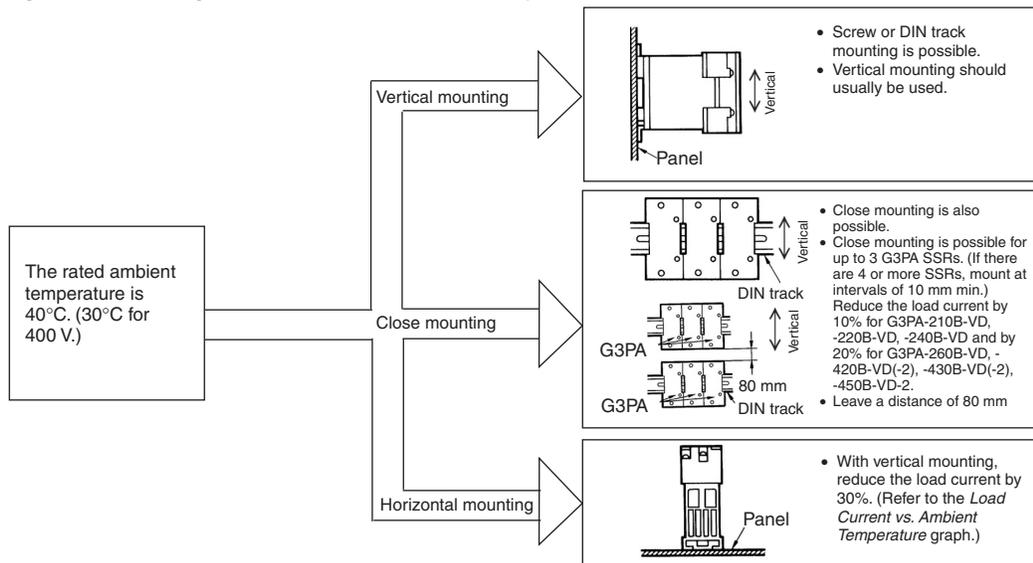
**Note:** Leave a distance of 60 mm min. between SSRs and ducts (especially above the SSR).
