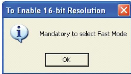
Figure 12. Pop up message for mandatory incremental setting when selecting 16-bit for absolute.
