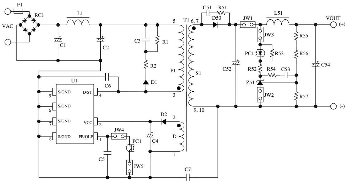
Figure 12-2 Circuit schematic for PCB circuit trace layout
