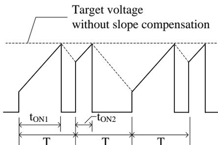
Figure 10-7 Drain current,  $I_D$ , waveform in subharmonic oscillation
