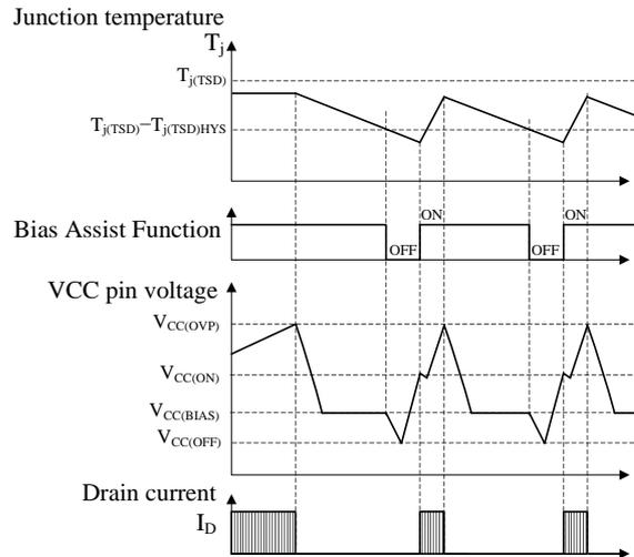
Figure 10-13 OVP operational waveforms at high temperature
