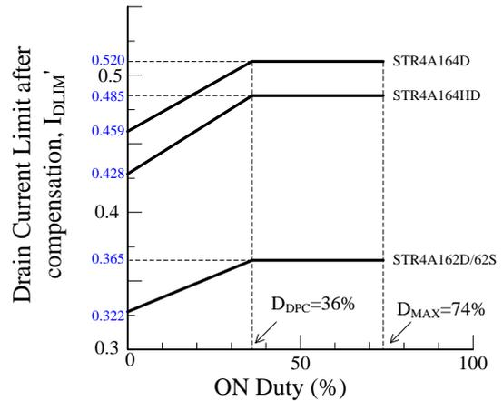
Figure 10-9 Relationship between ON Duty and Drain Current Limit after compensation
