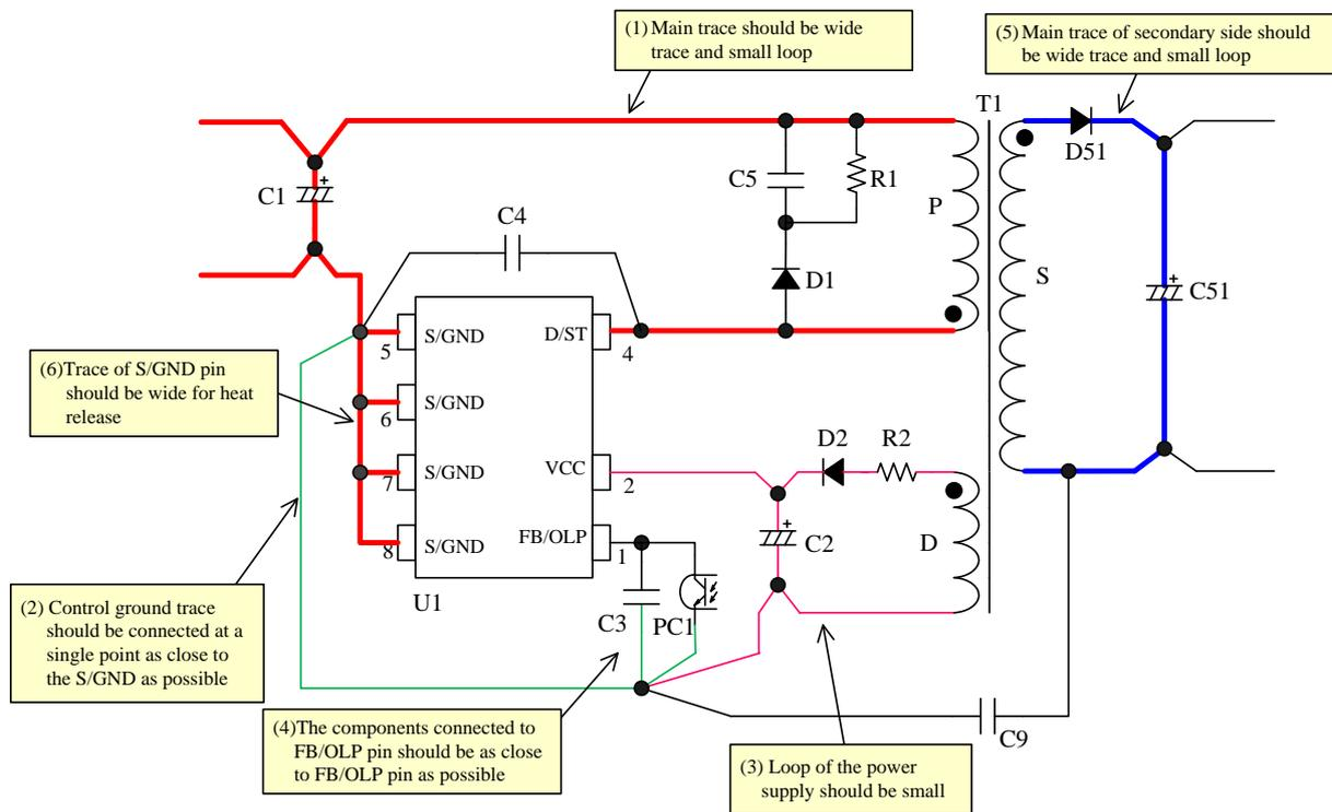
Figure 11-7 Peripheral circuit example around the IC
