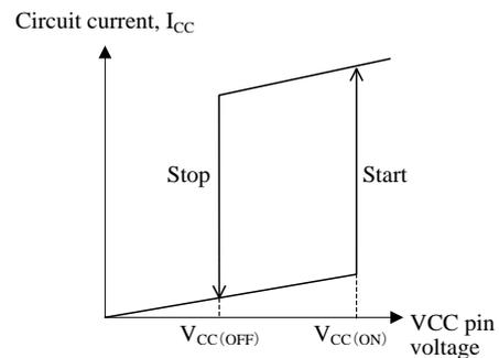
Figure 10-2 Relationship between VCC pin voltage and  $I_{CC}$
