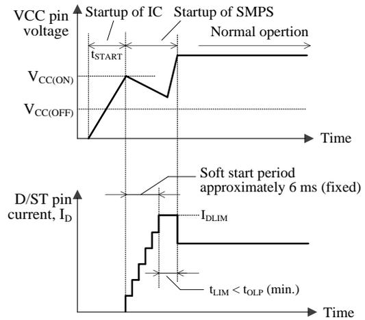
Figure 10-4 VCC and  $I_D$  behavior during startup
