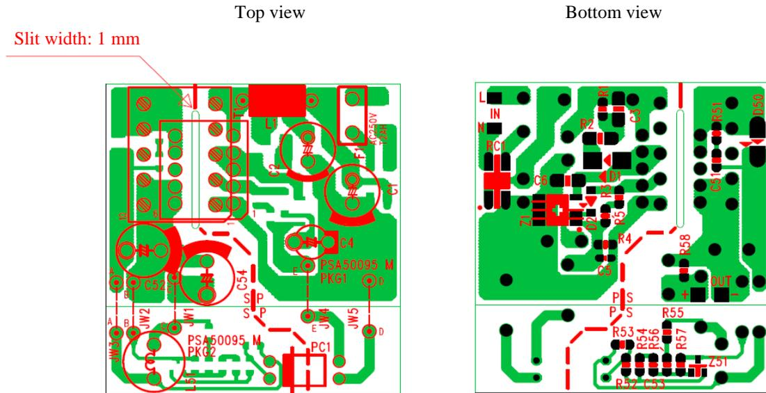
Figure 12-1 PCB circuit trace layout example (SOIC8 type)
