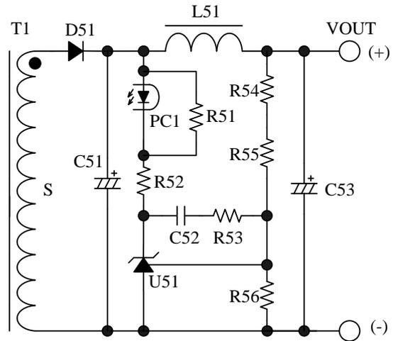
Figure 11-5 Peripheral circuit of secondary side shunt regulator (U51)
