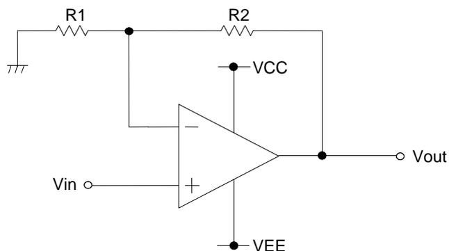
Figure 33. Non-inverting amplifier circuit
