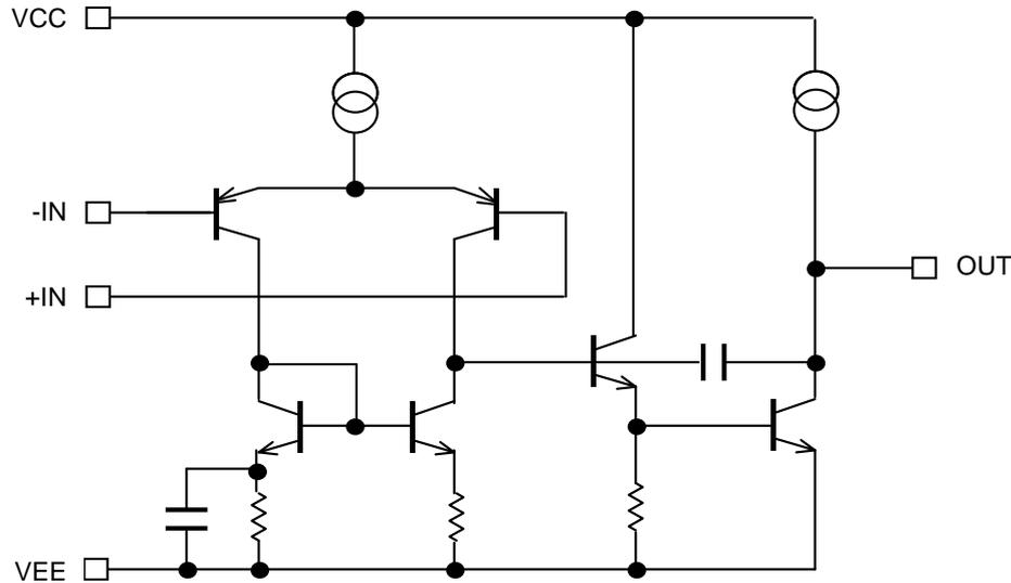
Figure 1. Simplified schematic
