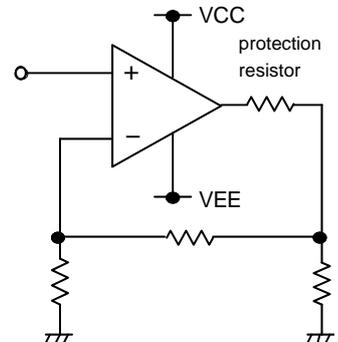
Figure 35. The example of output short protection
