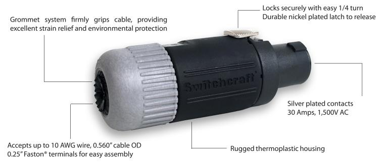
Switchcraft's HPC connectors are fully compatible with Neutrik® Speakon® connectors. Speakon® is a registered trademark of Neutrik®
