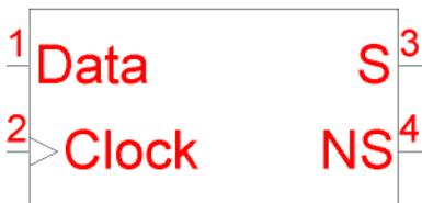
The new symbol will appear in the scheme, similarly to our example symbol shown at left. We can see our two 2 input pins and two output pins.
